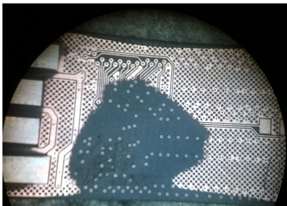
Example of monolith destroyed with too much sanding
