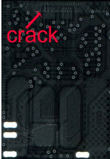
Example of X-ray view of a cracked monolith flash drive
