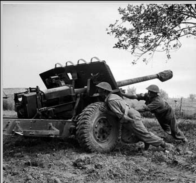
Gun crew of 267 Battery, 67 Anti-Tank Regiment, Royal Artillery prepare a 17 pounder Pheasant anti-tank gun for action
