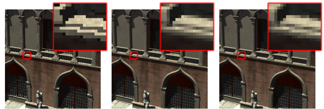
Fig. 8: We integrated anti-aliasing techniques into 3D rasterization: The rendering on the left uses the 3DR full algorithm (see Sect. 5) without any anti-aliasing, using 16 \times MSAA (center) takes 11 \times longer, while CSAA with 4 shading and 12 coverage samples (right) takes only 4.3 \times longer. Shading is computed using recursive ray tracing with 1 shadow ray, and 1 reflection ray for every sample.
