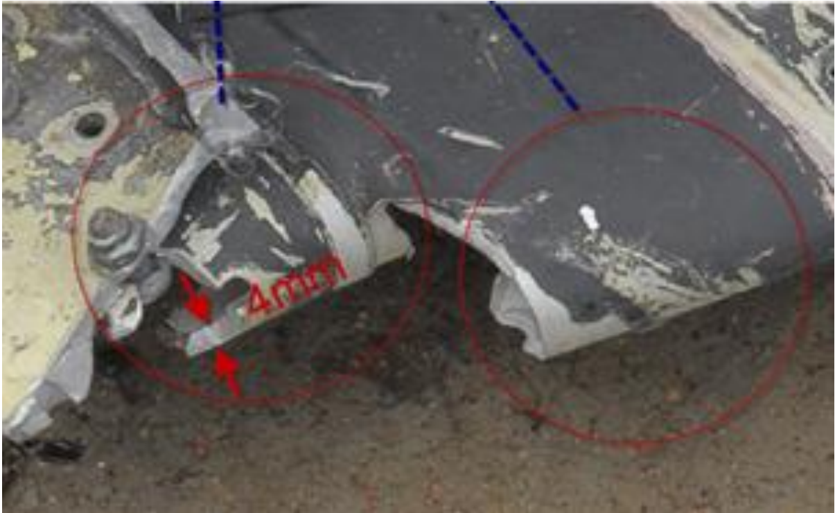
Fig. 22. A close-up of the photograph from Fig. 21 with visible post-shock curls with axis of curl in the direction of flight.
