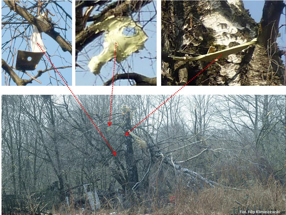
Fig. 4. Identified pieces of the detachable left wing part hanging on April 10, 2010 on the branches of (Bodin) birch tree claimed to have cut the wing (noted "bb").
