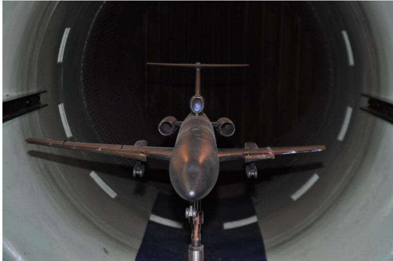
Fig. 25. Airplane model in the wind tunnel of the Institute of Aviation. Here in version with a cut left wing and without slats and the outer flap.
