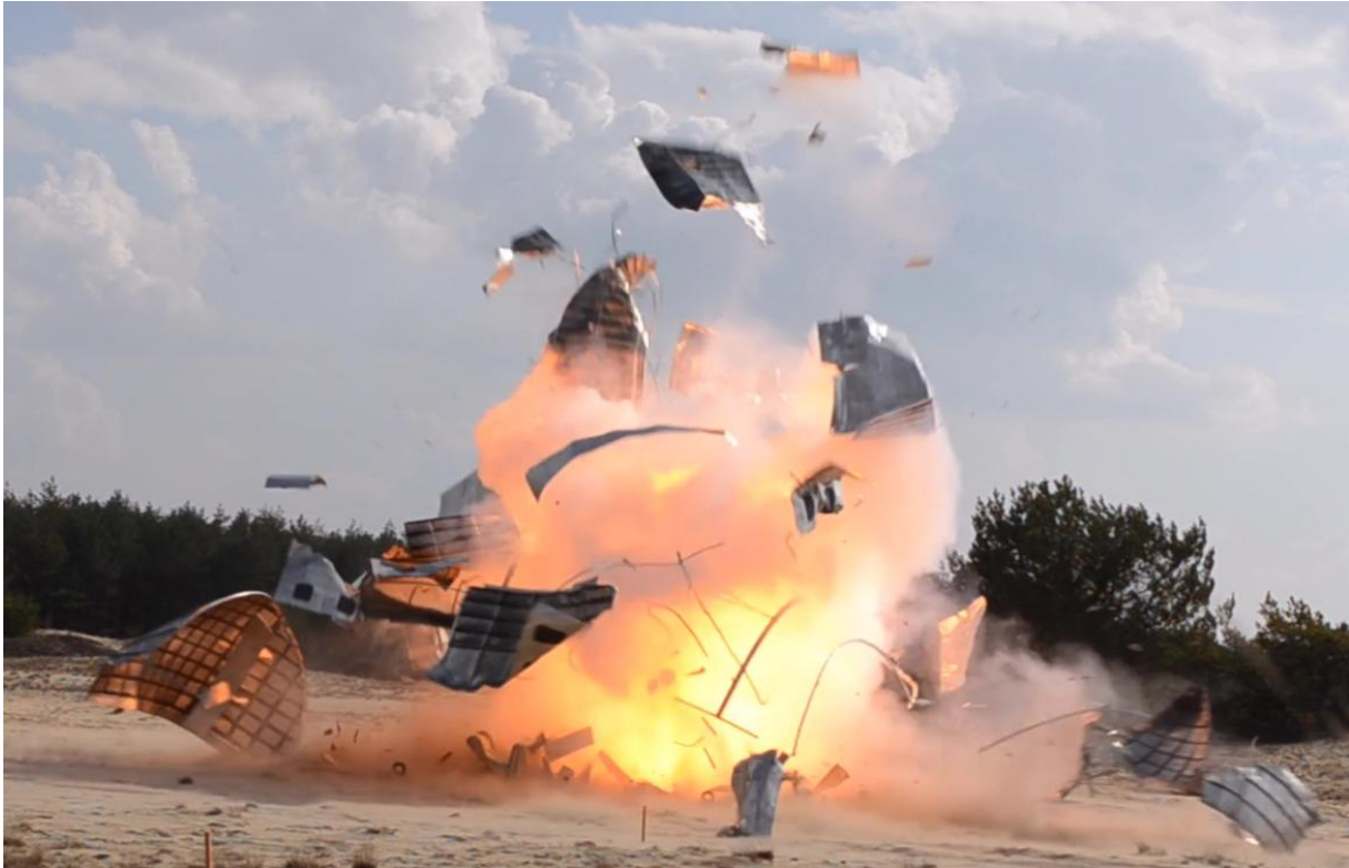
Fig. 52. Explosion of a thermo-baric charge in the occupant's part of the fuselage resulting in the complete destruction of the fuselage and the formation of a lot of small debris.
