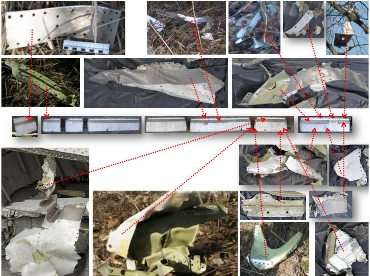
Fig. 16. Condition of the nose of the left wing according to the model reconstruction made by the Committee
