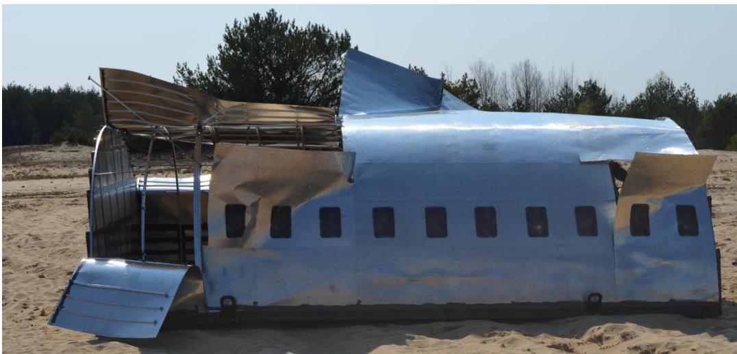
Fig.51. Explosion of jet-fuel in the occupant's part of the fuselage resulting in a large opening but not resulting in destruction into small pieces.
