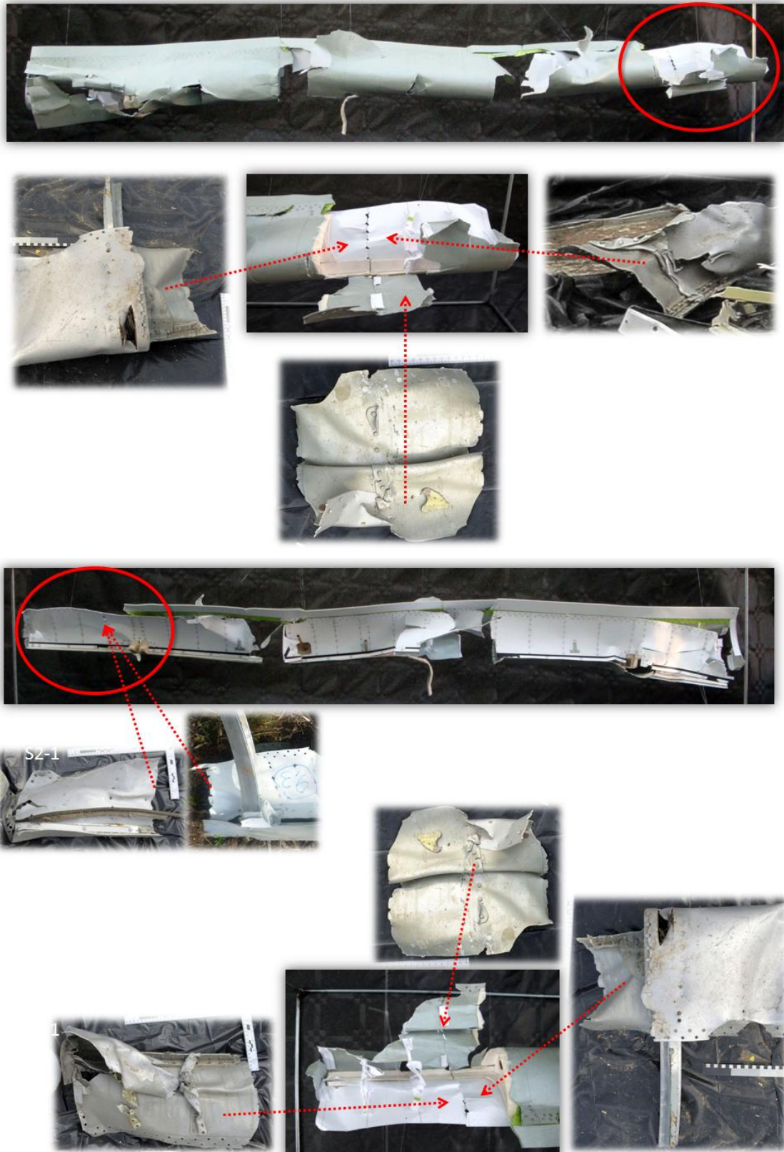
Fig. 17. Condition of the second section of the left wing slat according to the model reconstruction made by the Committee
