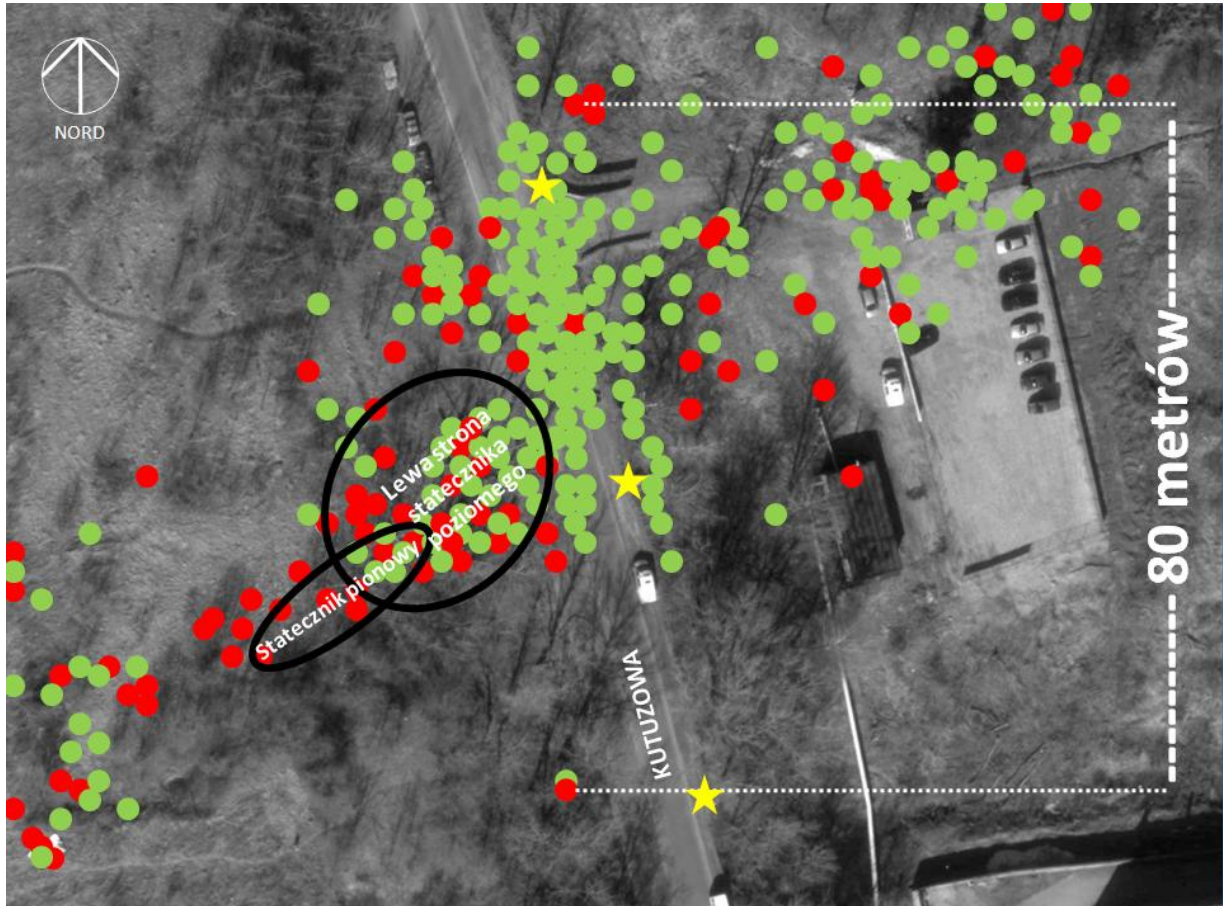
Fig. 27. Placing the left side of the horizontal stabilizer and the vertical stabilizer behind Kutuzov highway. Flight direction is from right to left. Red dots show debris from the Tu-154M and green dots show debris from the associated tree damage.
