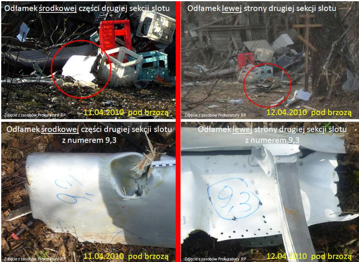
Fig. 19. Fragments of 2 sections of the slot moved from the original location on the ground under the tree claimed to have made contact with the wing.
