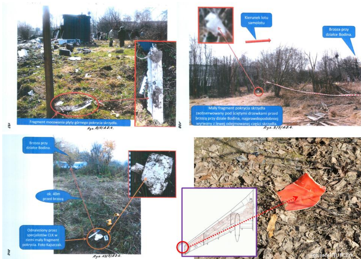
Fig. 3. Debris of the detachable part of the left wing identified by the Committee and experts of the Prosecutor's Office of the Republic of Poland.
