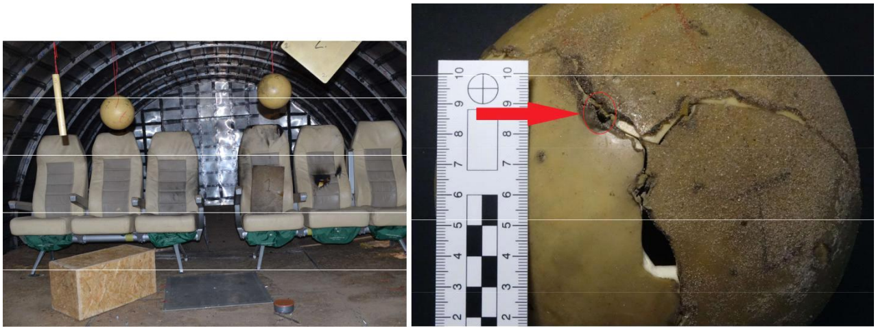
Fig. 53 Medical phantoms inside the model of the occupants part of the plane
