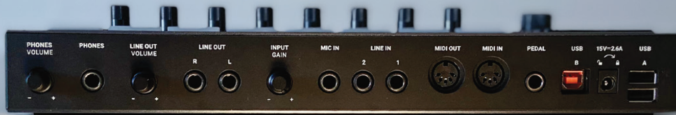
On the back panel we find stereo audio I/O, controls for headphone volume, line out volume and input gain, a pair of full-size MIDI ports, and three USB ports.
