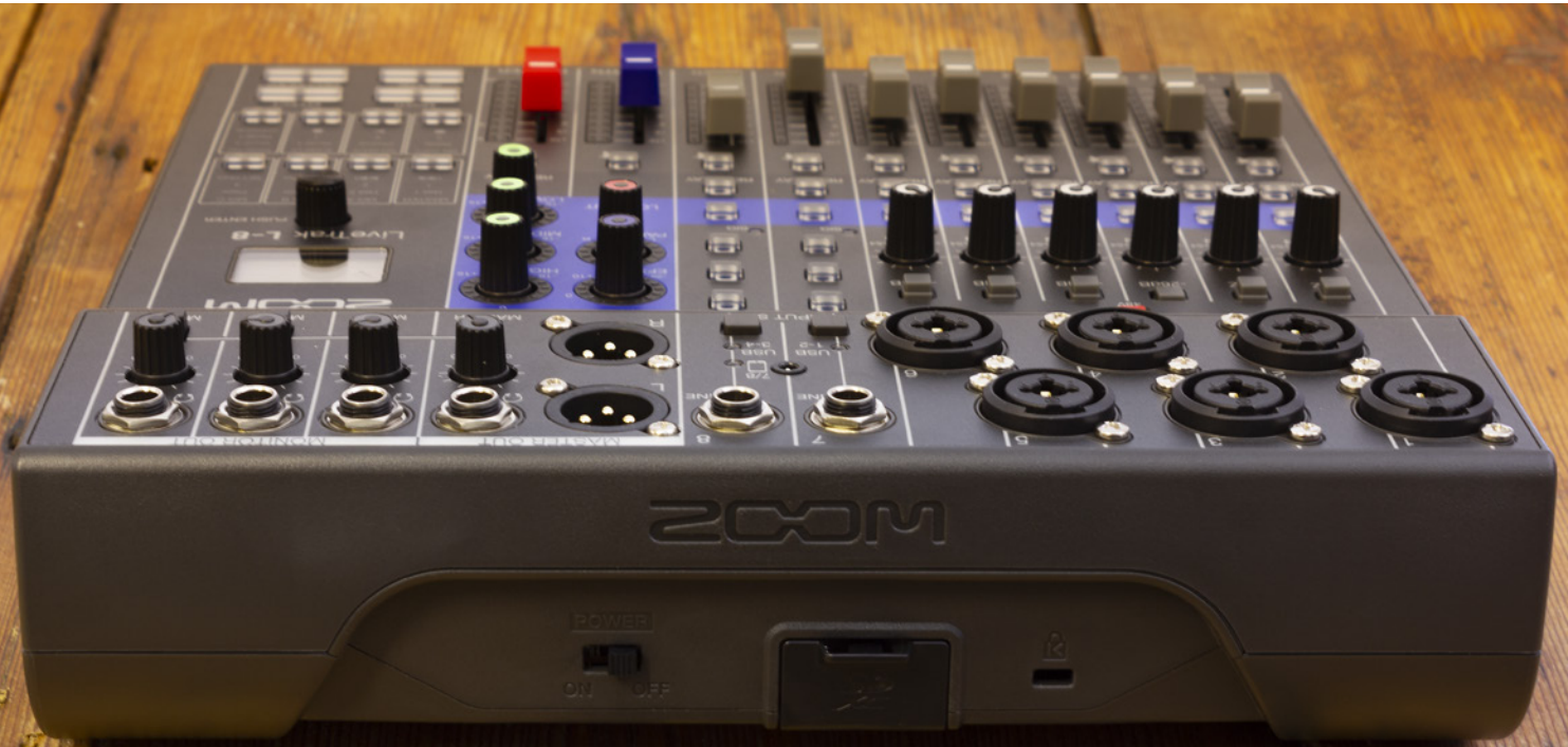
The SDHC/SDXC card for the multitracker recorder is inserted in a compartment at the rear, where you'll also find the on-off switch.
