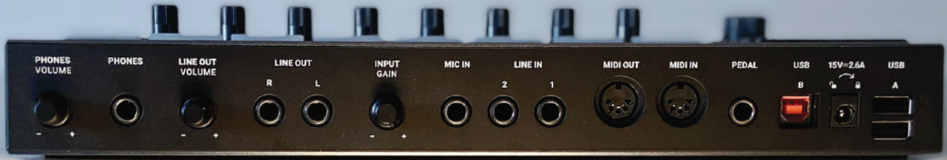
On the back panel we find stereo audio I/O, controls for headphone volume, line out volume and input gain, a pair of full-size MIDI ports, and three USB ports.
