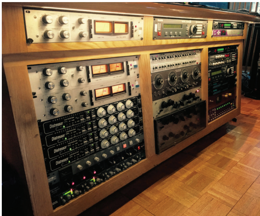
Bob Clearmountain's collection of outboard processors include a number of UREI 1178s, Empirical Labs Distressors, and various Eventide multi-effects units.
