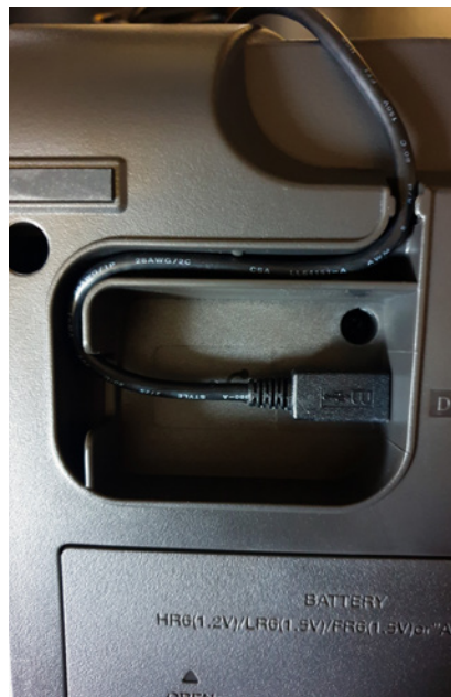
■ The USB 2.0 port, tucked beneath the L-8, has a good strain-relief system, and can be used for communication with and bus powering by a computer, or to hook up to the supplied mains power adapter or a USB battery. Alternatively, four AA batteries can power the L-8.
