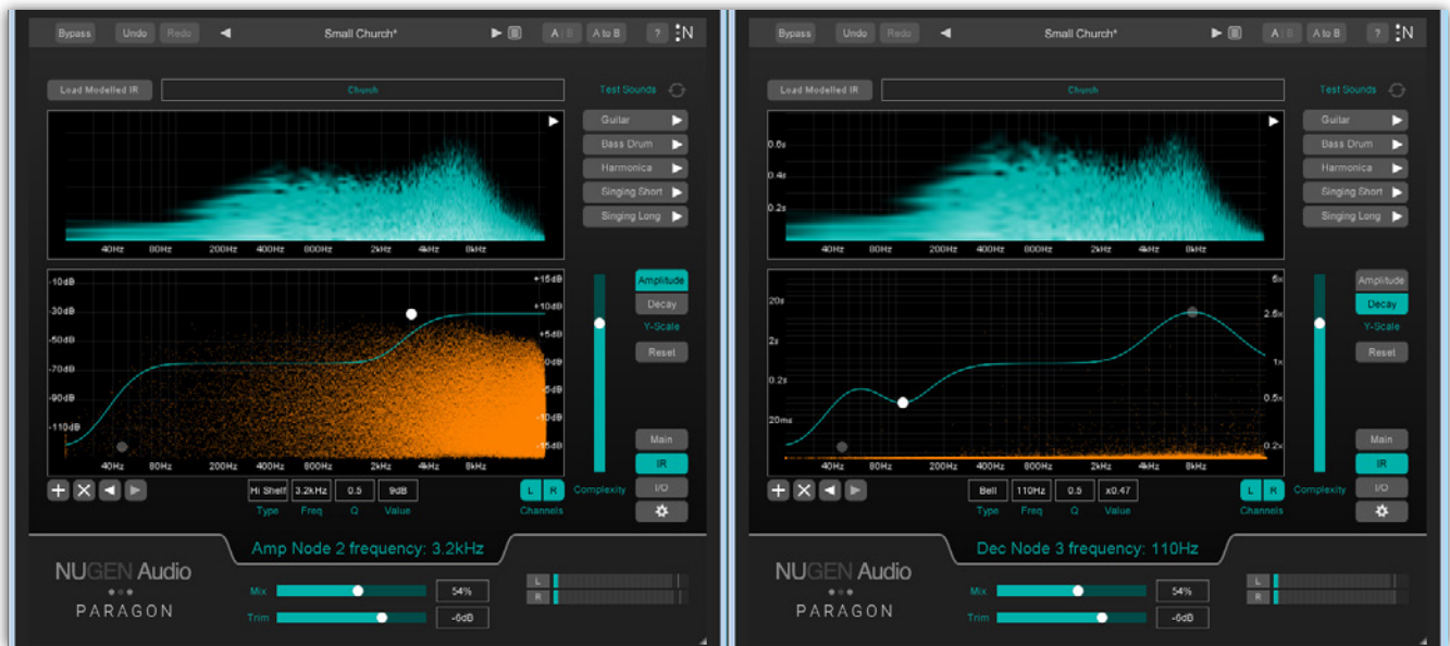
Both the amplitude (left) and decay (right) can be adjusted differently at different frequencies.
