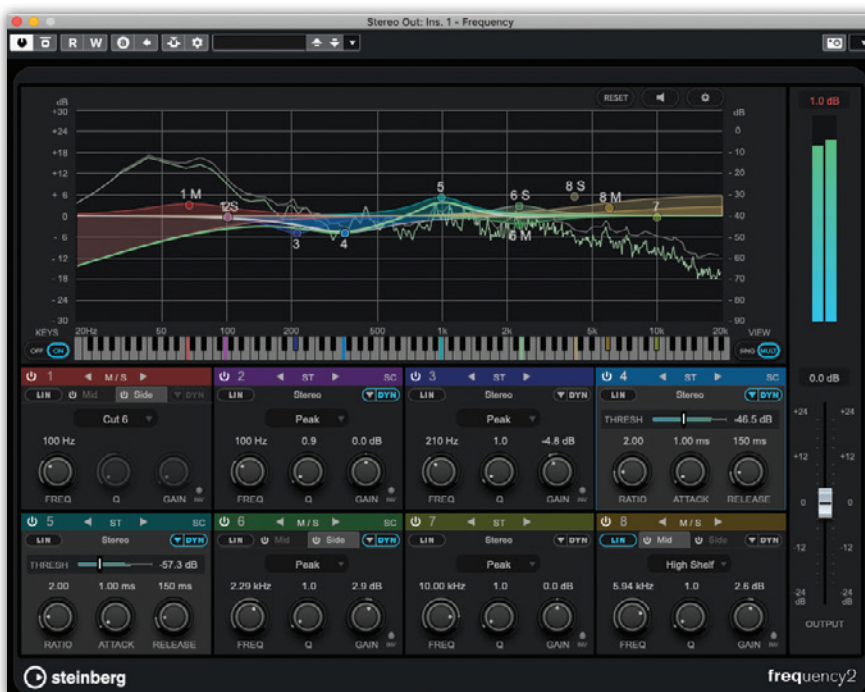
Frequency 2 adds dynamic EQ and multiple side-chain support to Cubase Pro's flagship EQ plug-in.
