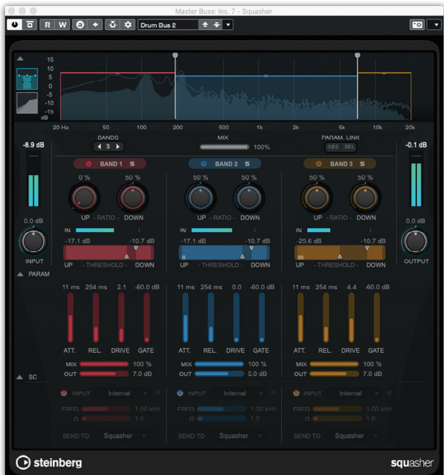
Squasher provides both downwards and upwards compression across three frequency bands and with support for multiple side-chain inputs.
