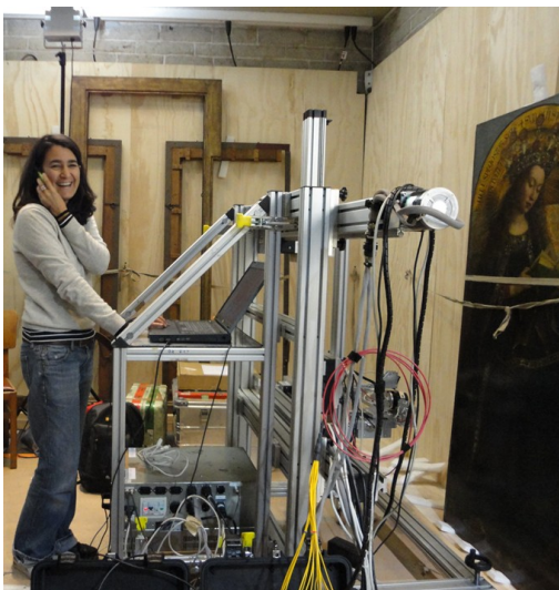
Fig. 18. Claudia Daffarra (INOA) and the multispectral IRR scanner at work on the Enthroned Virgin
