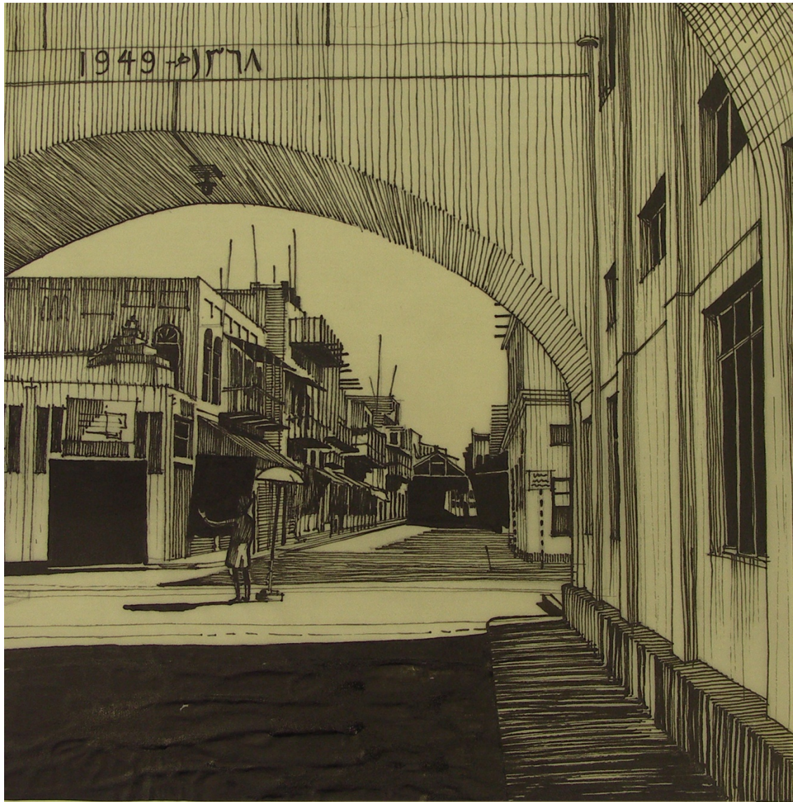
STREET SCENE ON BAHREIN ISLAND. The picture shows various method of providing shade, including masonry archways, balconies, projecting hoods and awnings, a roof covering the whole street, and an umbrella for the policeman. (Courtesy: Hunting Aerosurveys Ltd., London.) 3.12. B
