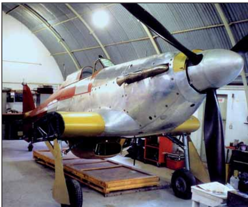
The Hawker Hurricane in the early stages of restoration
