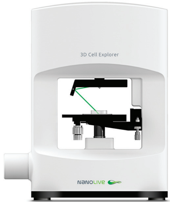
Figure 1: Marker-free 3D Cell explorer sample stage setup. The rotating scanning head illuminates the sample from all directions with a 520nm green laser light at low power.
