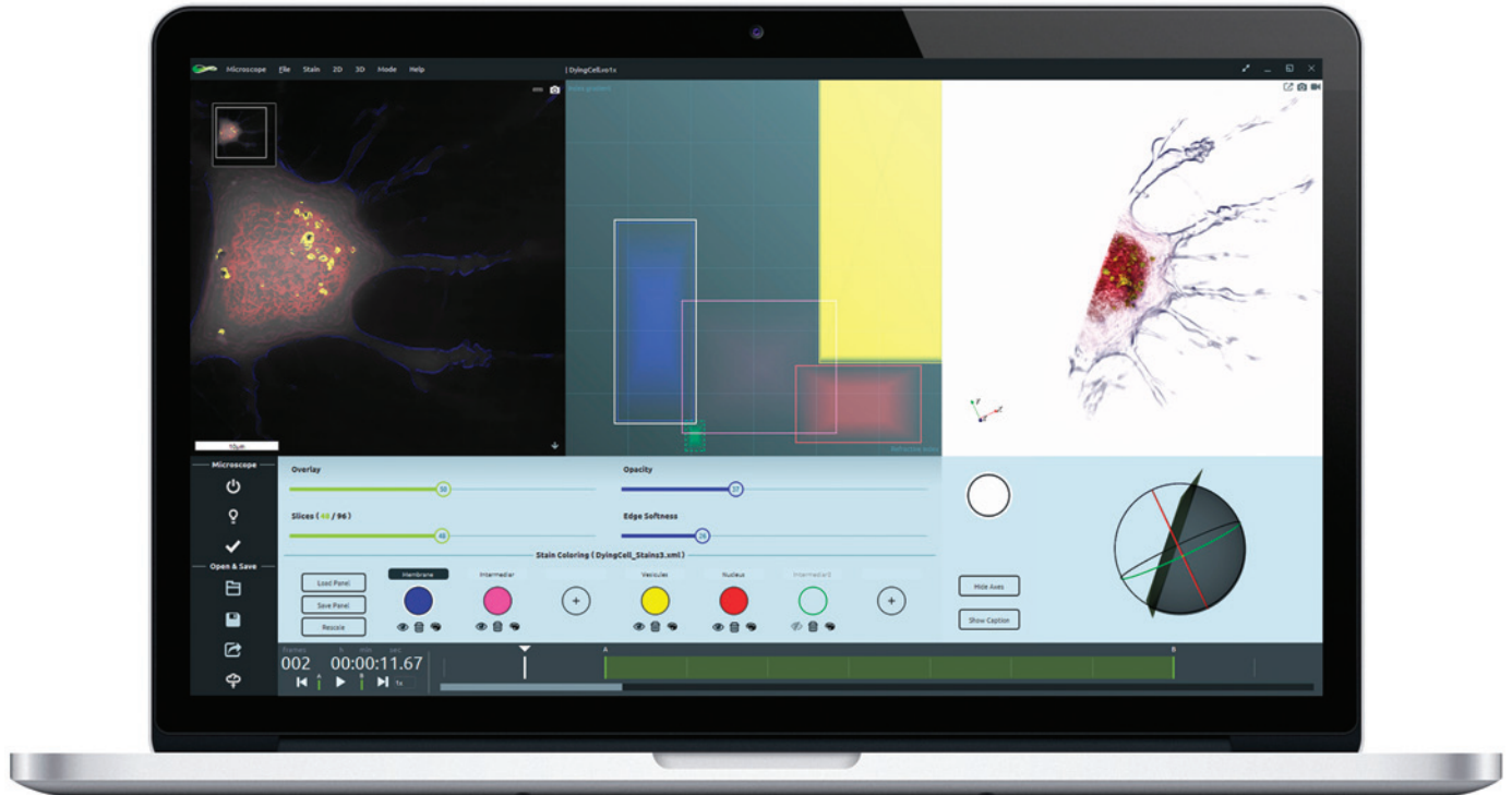
Figure 3: STEVE interface screenshot. The panel on the left offers a 2D viewer of the 96 z-stacks that compose the 3D image on the right. In the center, the Panel Viewer constitutes a fingerprint of the analyzed cell. In the x-axis refractive indexes are reported, while the y-axis shows the gradients. On the bottom (Control Field) the user can choose the color to apply to each cell part in order to produce the 3D reconstruction and modulate its transparency.
