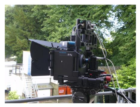
Figure 1: A photograph of the P+S Technik mirror rig, shown here equipped with Silicon Imaging SI-2K Mini camera heads (right and, partially concealed, on top). Also visible are a P+S Technik 3d sync box (mounted top right) powered by a camera battery (resting on top of the rig, in front of the top camera), which provides timing information to synchronise the cameras.
