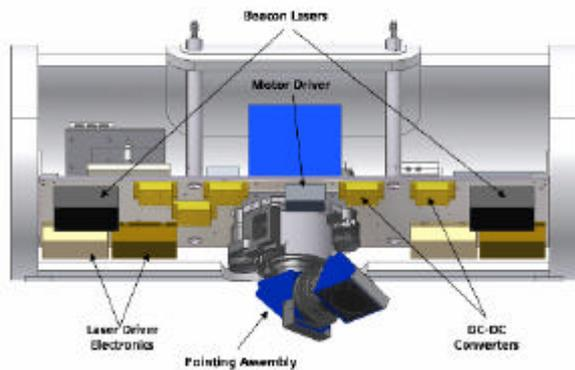
Fig. 4. CAD sketch of FELT – Bottom side.
