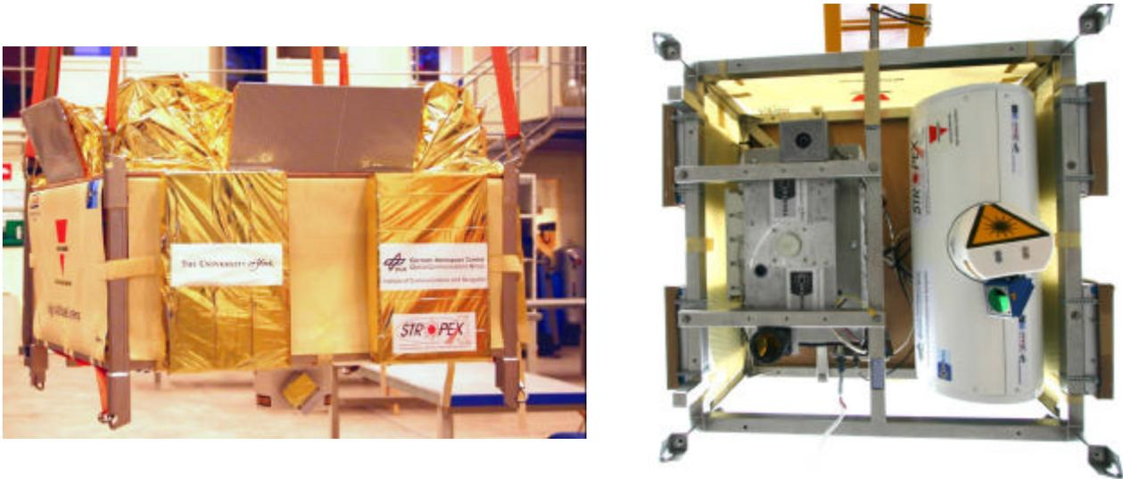
Fig. 10. Integrated CAPANINA payload. Millimeter-wave and optical payload (FELT) integrated into the nacelle. Front view (left) in the integration room and bottom view on the launch vehicle (right). Retro reflectors are attached at the top of the payload which is also covered with solar radiation protection foil.
