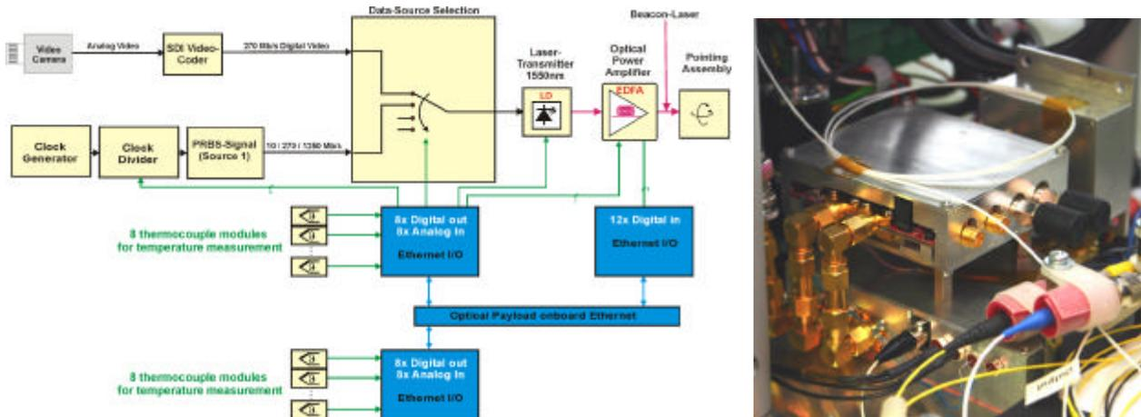
Fig. 7: Block diagram of FELT Data electronics (left) and photo of the system during integration into the FELT (right). The upper housing with the wound-up fiber on top is the pseudo random binary sequence generator mounted on top of the data source selection and laser transmitter module. The vertical housing in the background is the Clock generator.
