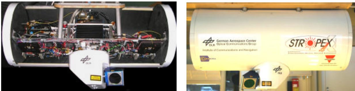
Fig. 3. Assembly photo of FELT with opened carbon fiber housing (left) and the ready to fly terminal (right) before payload integration.
