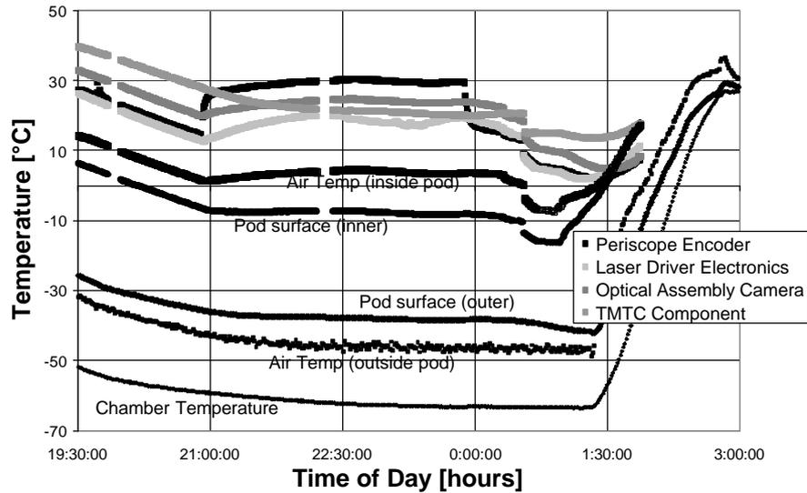
Fig. 9. Selected FELT thermocouple data from the thermal vacuum chamber test
