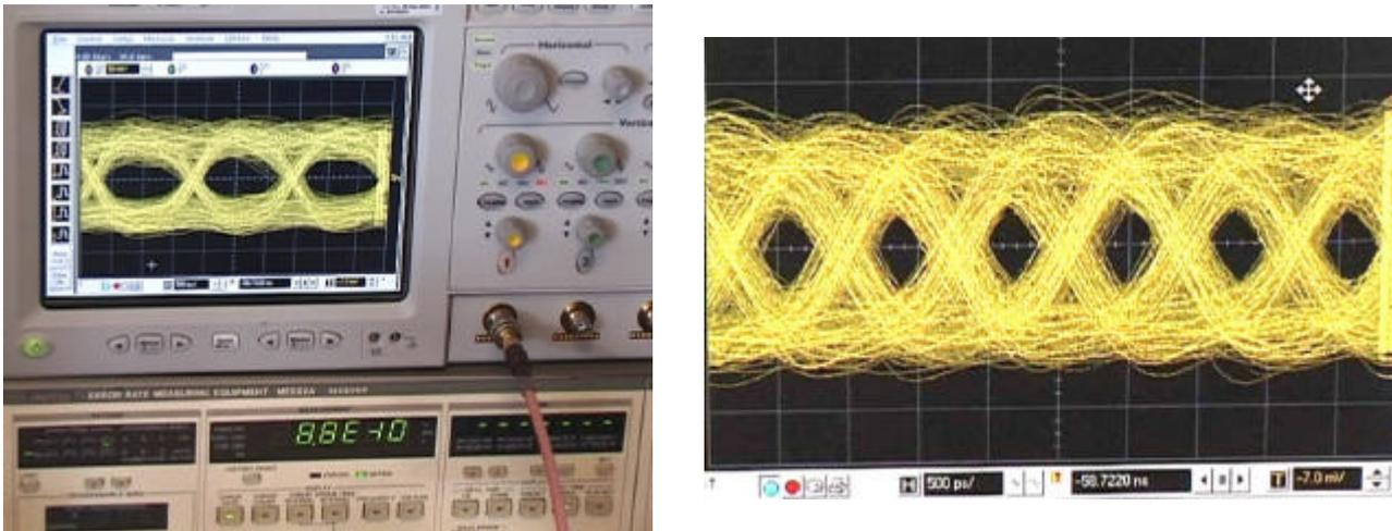
Fig. 16: Received signal PRBS eye patterns. 622 Mbit/s eye pattern with bit error rate measurement receiver (left picture) and 1.25 Gbit/s eye pattern (right picture) at approximately 60 km range.
