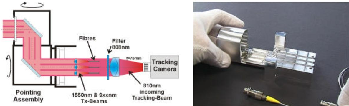
Fig. 6: Schematic sketch of optical assembly with pointing assembly (left) and one of the machined optical assembly prototypes during the assembly of fibres (right)
