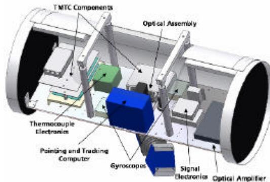
Fig. 5. CAD sketch of FELT – Top side.
