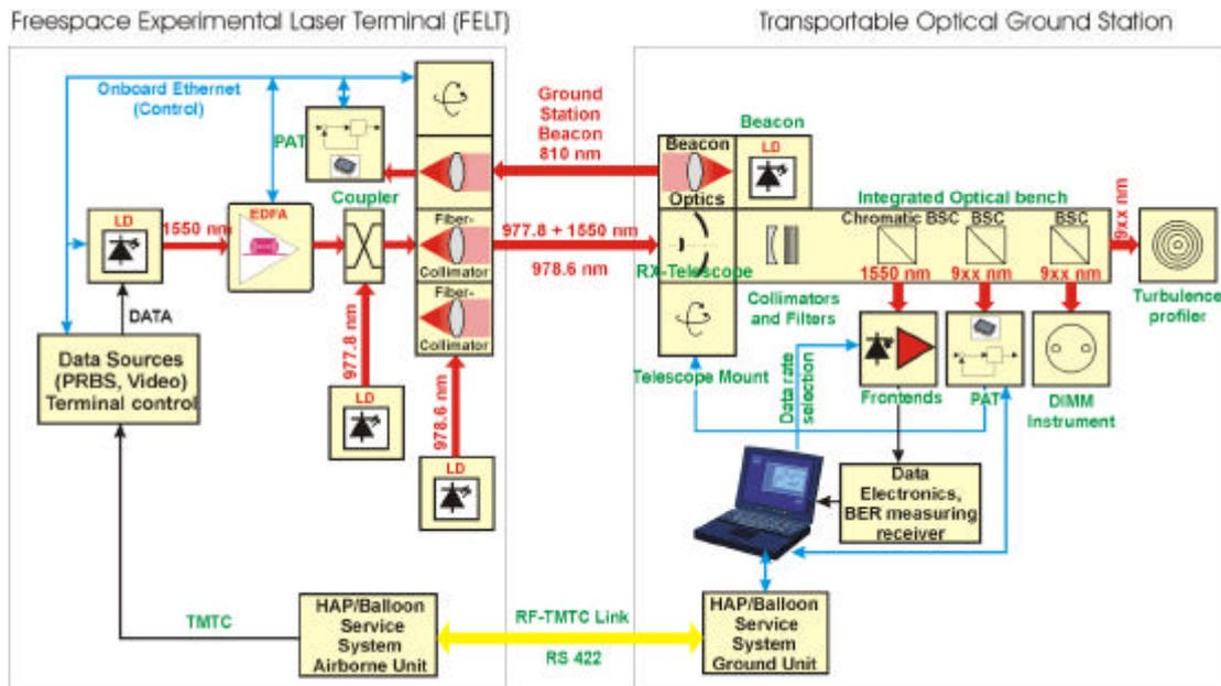
Fig. 2. Block Diagrams of the FELT and TOGS
