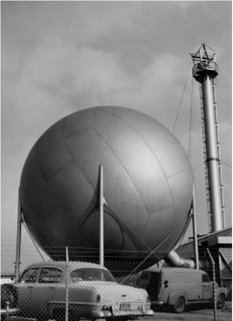
The sphere at the Freeport Laboratory in Long Island enabled Poly professors to produce high-speed airflow, simulating conditions of supersonic aircraft while in flight. This research further fueled the U.S. space program.
