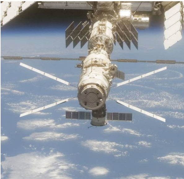
Rear view of ATV docked to the ISS on with clear view of cross-shaped solar arrays. (Image: NASA)
