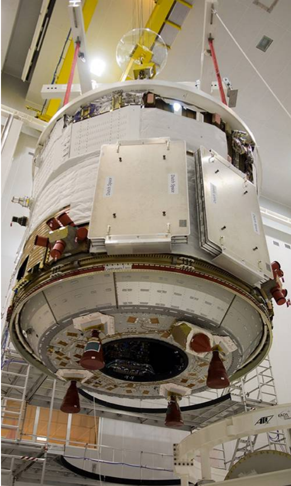
The ATV Service Module being hoisted into position for mating with the Integrated Cargo Carrier on 12 December 2007. Two solar panels shown folded up. (Image: ESA /CNES/Arianespace/Photo optique video du CSG)
