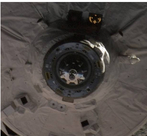
ATV docking mechanism during Demonstration Day 2 in orbit, when it was brought to within 11 metres of the ISS on 31 March 2008. (Image: NASA)
