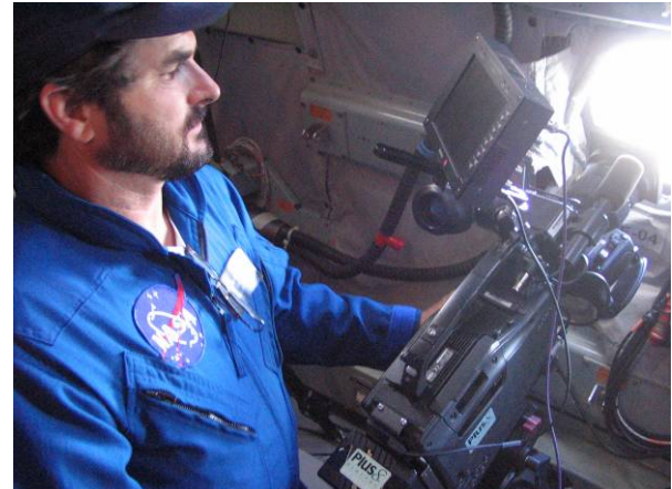
HDTV spectrograph during the Genesis capsule re-entry observation campaign in 2004. (Image: NASA Ames Research Center)
