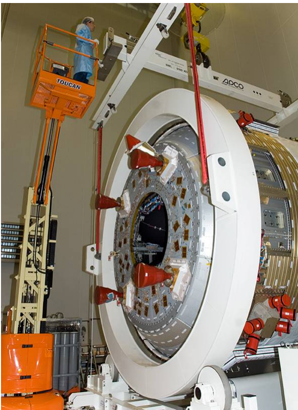
End of the ATV propulsion bay clearly showing four main thrusters and one complete attitude control thruster cluster (lower right) covered with red protective caps. Photo taken on 13 December 2007. (Image: ESA /CNES/Arianespace/Photo optique video du CSG)
