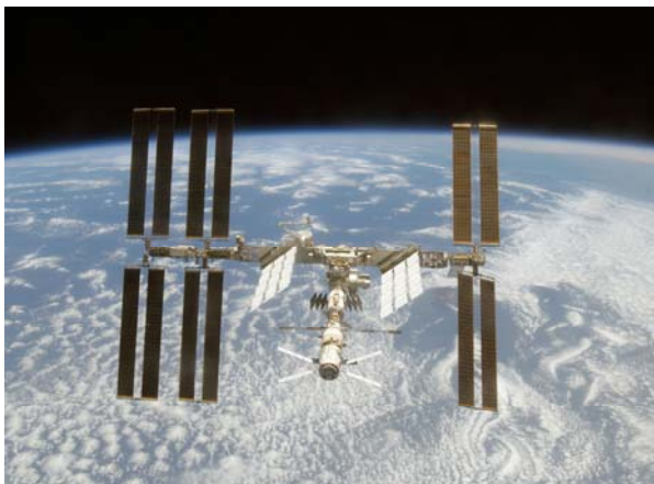
For undocking the Station will be tilted by a few degrees, front to back, with the ATV situated at the back of the Station. (Image: NASA)
