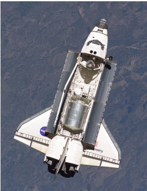
Multi-Purpose Logistics Module (MPLM) in Shuttle cargo bay during docking of STS-121 Discovery mission on 6 July 2006. The flight also brought ESA astronaut Thomas Reiter to the ISS to serve as the first European ISS Expedition crew member. The ATV Integrated Cargo Carrier is based on the MPLM. (Image: NASA)
