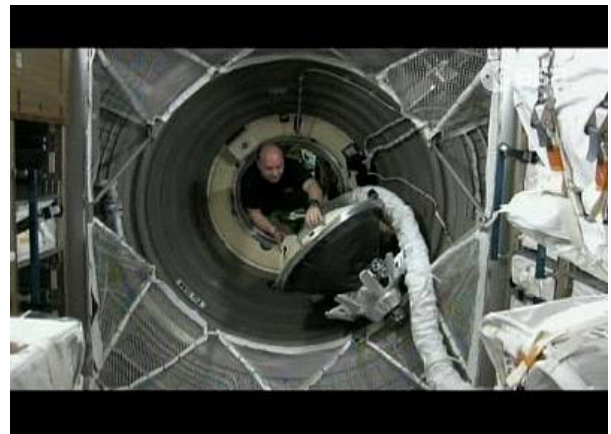
NASA astronaut and Expedition 16 Flight Engineer Garrett Reisman entering the ATV past the ATV docking mechanism and inter-module air hose (Image: ESA TV)
