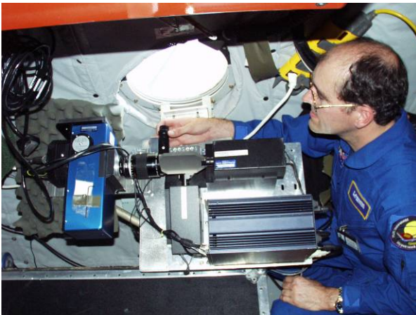
AIMIT tracker and Echelle slit spectrograph during the Genesis capsule re-entry observation campaign in 2004. These instruments will be used during the ATV re-entry campaign. (Image: NASA Ames Research Center)
