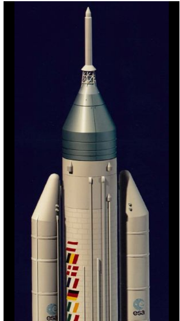
Artist's impression of the crew version of the Advanced Re-entry Vehicle in launch configuration on an Ariane 5. The spacecraft is in its fairing with a crew escape system located at the top of the stack (image: ESA/D. Ducros)
