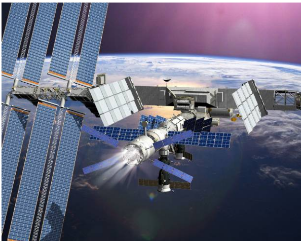
Artist's impression of the ATV reboosting the International Space Station to a higher orbiting altitude. (Image: ESA/D. Ducros)
