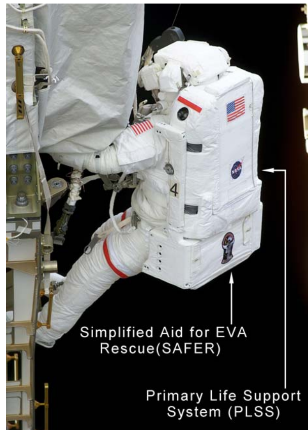
NASA Astronaut Michael Gernhardt in Extravehicular Mobility Unit during ISS spacewalk on the STS-104 mission on 21 July 2001. (Image: NASA)
