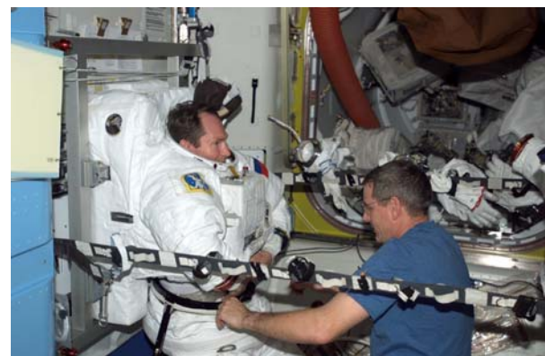
ISS Expedition 12 Flight Engineer Valery Tokarev being assisted into the Hard Upper Torso section of an EMU by Expedition 12 Commander Bill McArthur on 23 October 2005. (Image: NASA)
