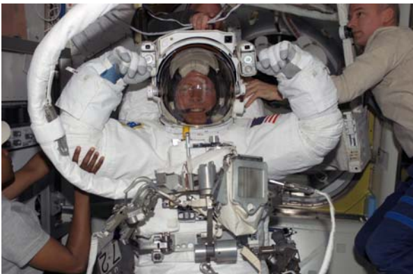
Top: Expedition 13 Flight Engineer Jeff Williams holding the Simplified Aid for EVA Rescue (right in picture) prior to attachment. Bottom: STS-121 Mission Specialist Michael Fossum, holds arms aloft as SAFER unit is attached to his EMU by STS-121 Mission Specialist Stephanie Wilson and Jeff Williams. (Image: NASA)
