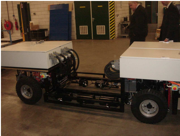
Figures 7 and 8. MASDAR Phase 1A Chassis Prototype "Workhorse" and Suspension Systems
