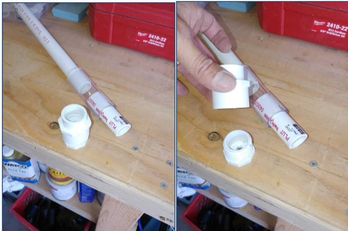
Photograph 8. PVC posts showing construction and individual pieces
