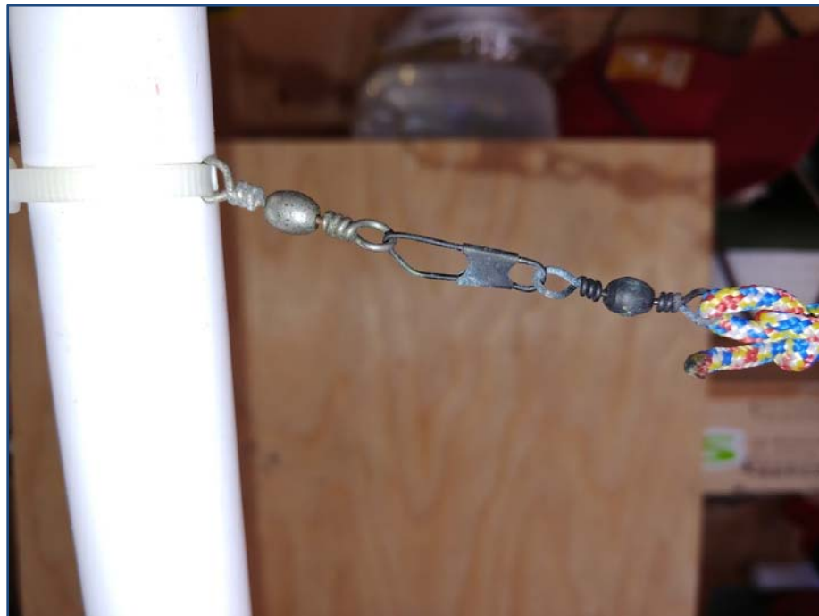
Photograph 9. Lines attached to PVC poles using zip ties and swivels
