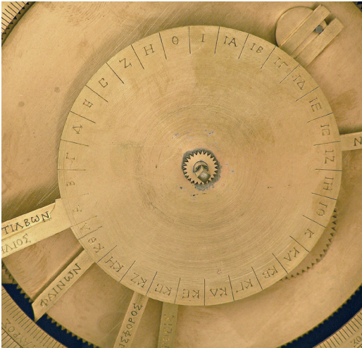
Fig. 12. Antikythera Mechanism, author's reconstruction. Centre of front dial with Moon-phase indicator removed.
