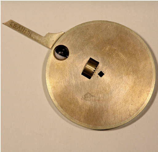
Fig. 10. Antikythera Mechanism, author's reconstruction. Moon-phase indicator, detached.
