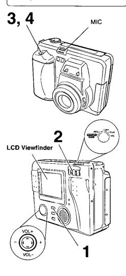
Press REC MODE repeatedly to select Motion (EE) or Burst ( ) recording mode.
