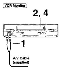
Connect the A/V OUT Terminal on the Camera and the AUDIO IN/VIDEO IN on the VCR or TV using the A/V Cable (supplied).
