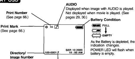
Displayed Image Page and its captured mode SF(Super Fine), F(Fine), N(Normal), or (III) (Motion Image Rec Mode).
