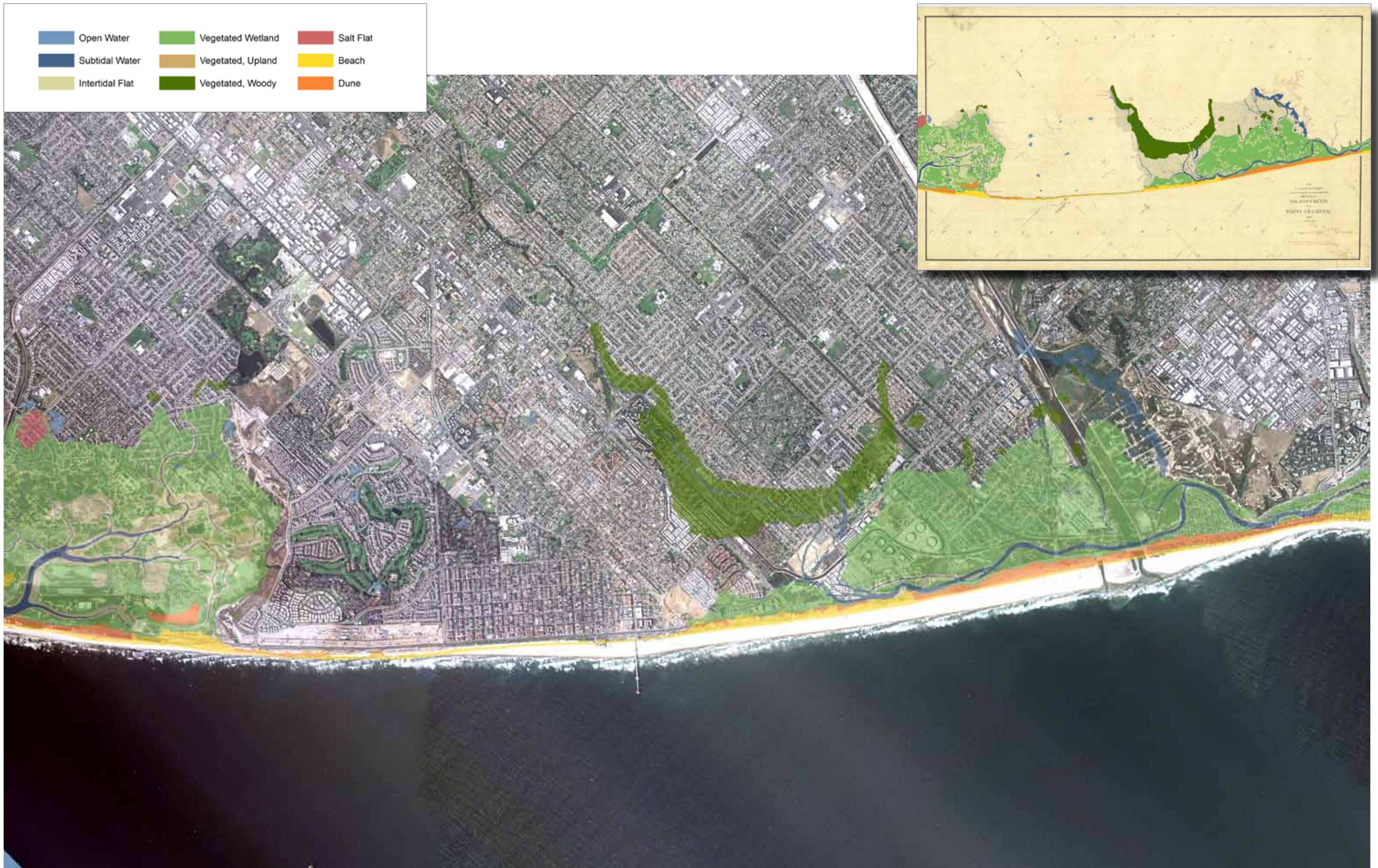
Figure B21. Coastal features digitized from T-1369, overlaid on modern aerial photography (USDA 2005), at same scale as facing T-sheet.
