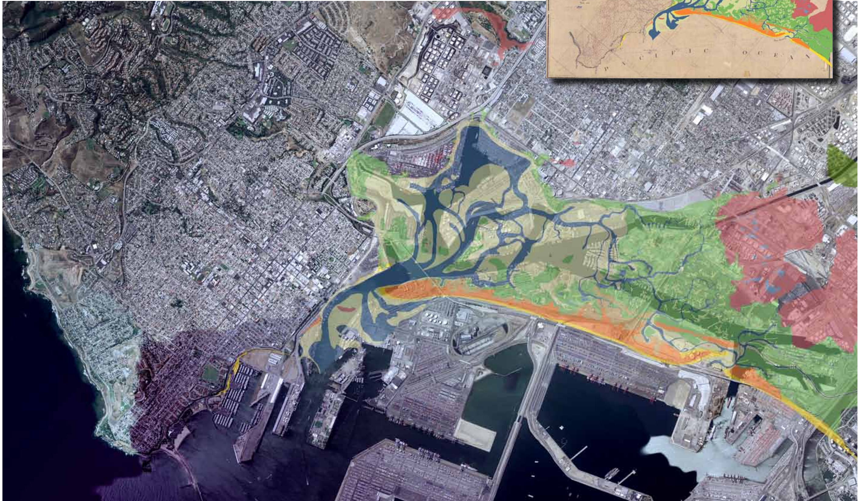
Figure B17. Coastal features digitized from T-892, overlaid on modern aerial photography (USDA 2005), at same scale as facing T-sheet.
