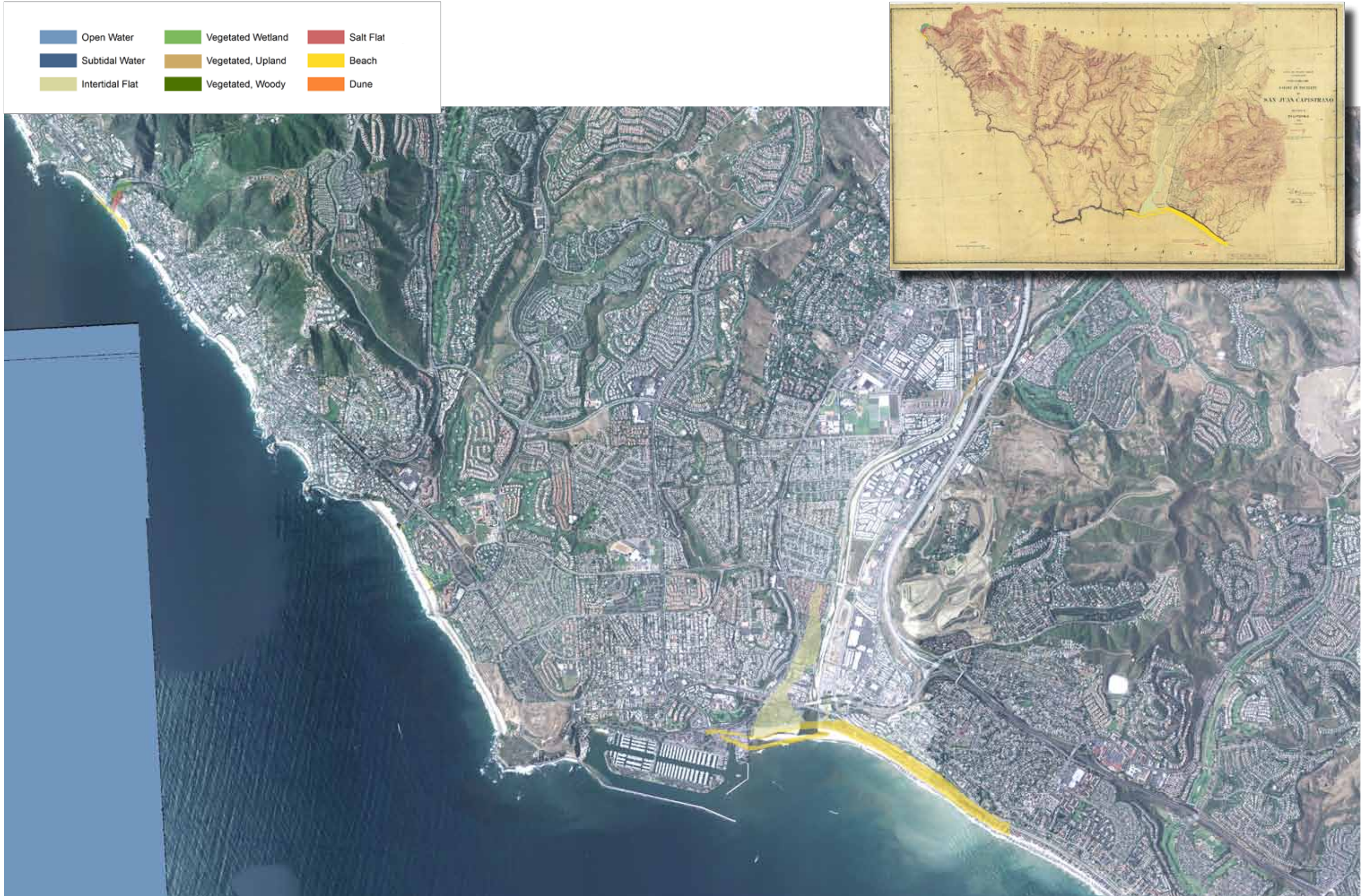
Figure B25. Coastal features digitized from T-1645, overlaid on modern aerial photography (USDA 2005), at same scale as facing T-sheet.
