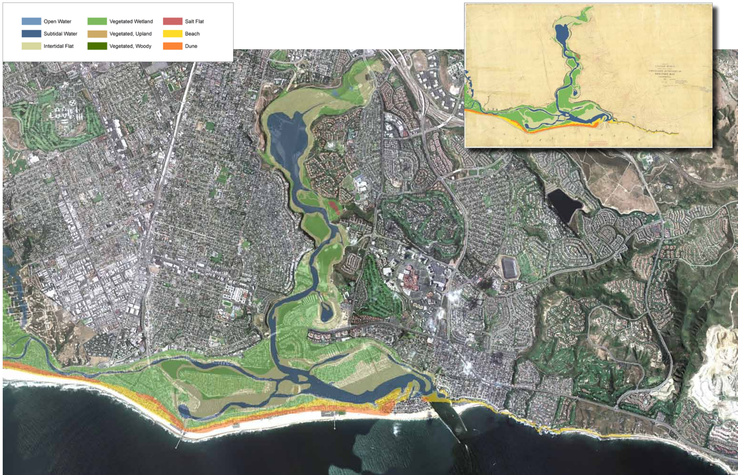
Figure B23. Coastal features digitized from T-1392, overlaid on modern aerial photography (USDA 2005), at same scale as facing T-sheet.
