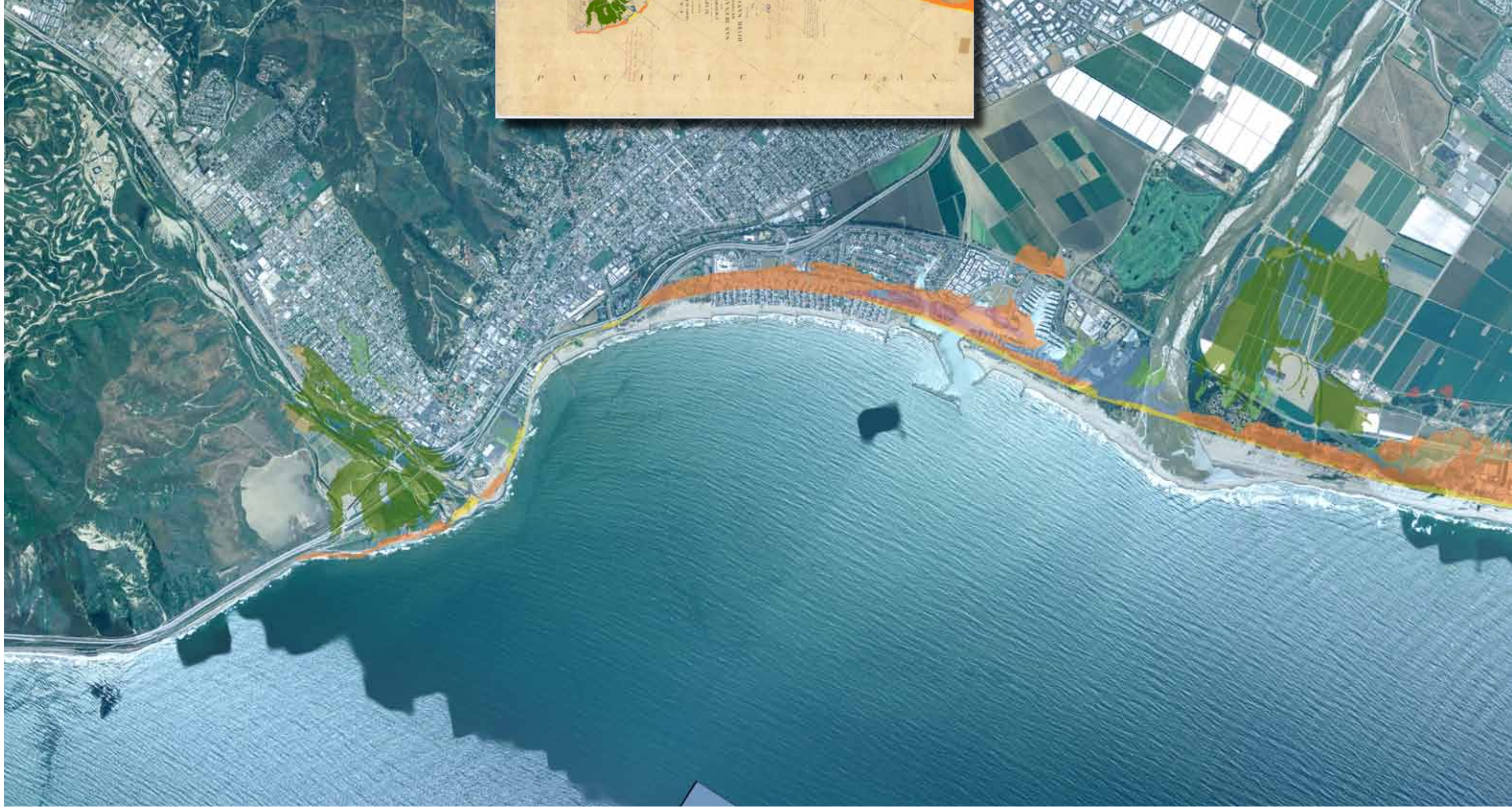
Figure B13. Coastal features digitized from T-683, overlaid on modern aerial photography (USDA 2005), at same scale as facing T-sheet.
