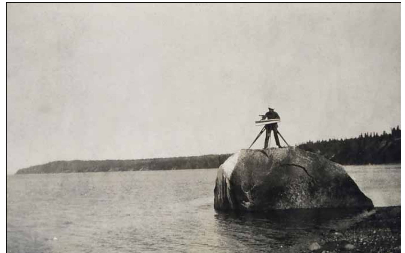
Figure 3. Coast Survey plane table mapping. The surveyor is using the plane table on an offshore rock in Cook Inlet, Alaska, circa 1910. The alidade can be seen on top of the surface of the plane table. (U.S. Coast and Geodetic Survey ca. 1910, courtesy of NOAA photo library)
