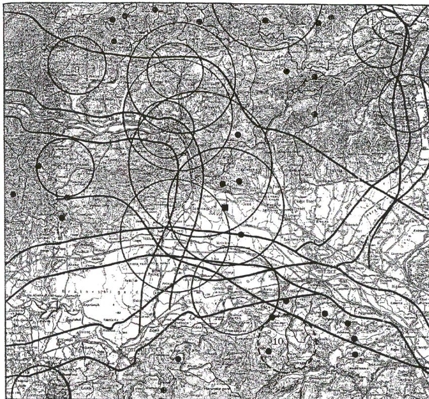
Fig. 7.6 Map of the seismic network region with all potential station sites (full dots) and known seismic noise sources (roads, railway, cities, villages, industrial facilities, quarries, etc) with circles of minimum recommended distances drawn around them for the case of gain 25.000 for SP seismic stations at 1 Hz set on hard clay, hardpan and similar ground, i.e., case
