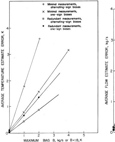
Fig. 6. Errors in temperature estimates for recycle network with measurement bias.
