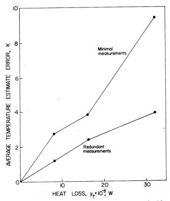
Fig. 5. Errors in temperature estimates for blending network with heat leak.
