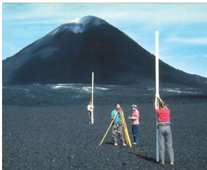
Leveling survey to determine changes in the ground surface relative to earlier measurements of the same surface. Young Pu'u 'Ō'ō cone looms up in the background.
