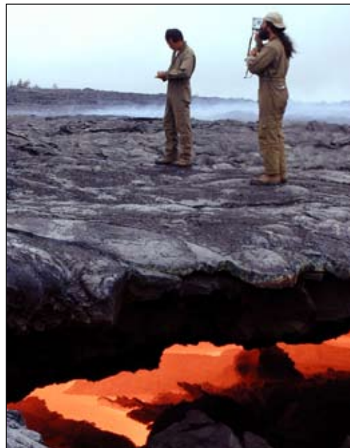
Jim Kauahikaua measures the electrical conductivity of the subsurface using a VLF (very low frequency) conductivity tool to determine the location of lava tube.
