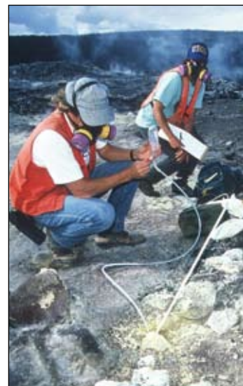
Jim Kauahikaua measures the electrical conductivity of the subsurface using a VLF (very low frequency) conductivity tool to determine the location of lava tube.
