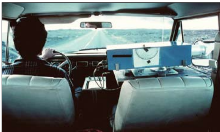
Vehicle drives beneath plume as COSPEC instrument sticks out the window, facing upward measuring sulfur dioxide concentrations. In the overhead volcanic plume. COSPEC measures light coming into the instrument after passing through the plume
