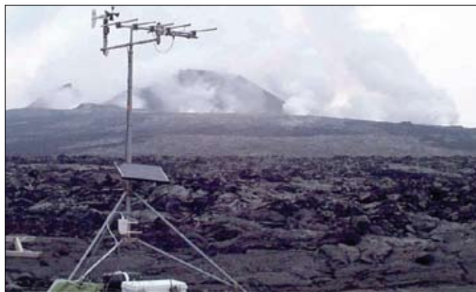
A small computer at this gas monitoring site located near Pu'u 'Ō'o (in background). Chemically-selective sensors for SO 2 and CO 2 measure gas concentrations and a wind sensor measures wind speed and direction. Data are transmitted to HVO every 10 minutes, providing near real time data on degassing from Pu'u 'Ō'o.
