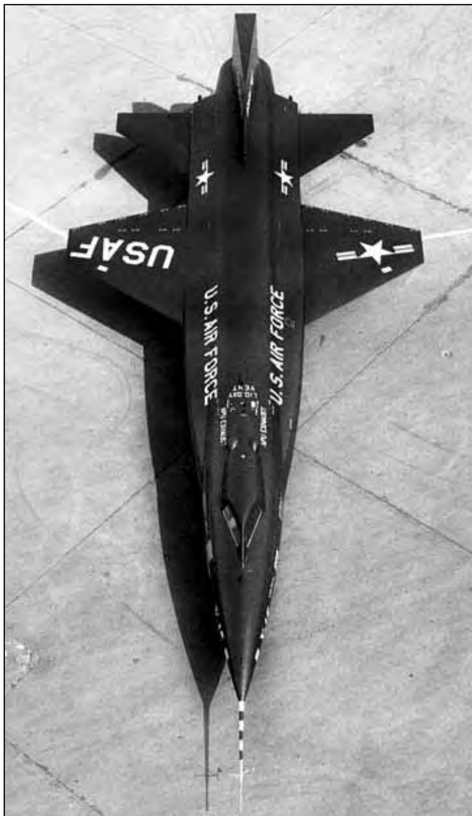
The first X-15 (56-6670) immediately prior to the official roll-out ceremonies at North American's Los Angeles plant on 15 October 1958. The small size of the trapezoid-shaped wings and the extreme wedge section of the vertical stabilizer are noteworthy. (North American Aviation)
