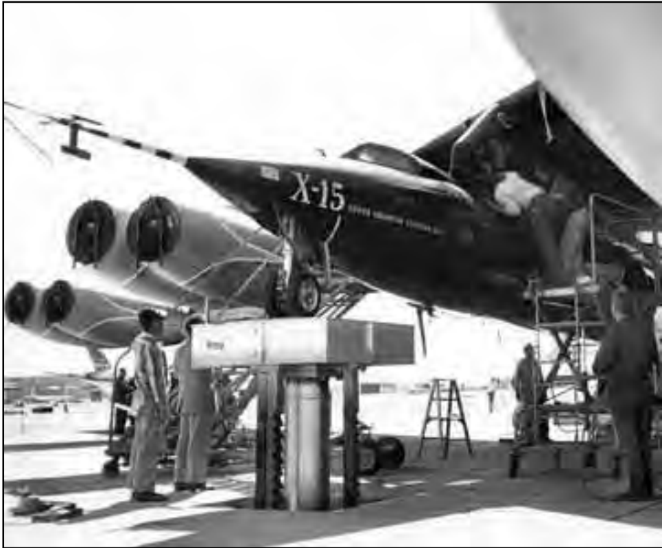
Hydraulic lifts were installed in the ramp at the Flight Research Center (now the Dryden Flight Research Center) to lift the X-15 up to the wing pylon on the NB-52 mothership. (Jay Miller Collection)
