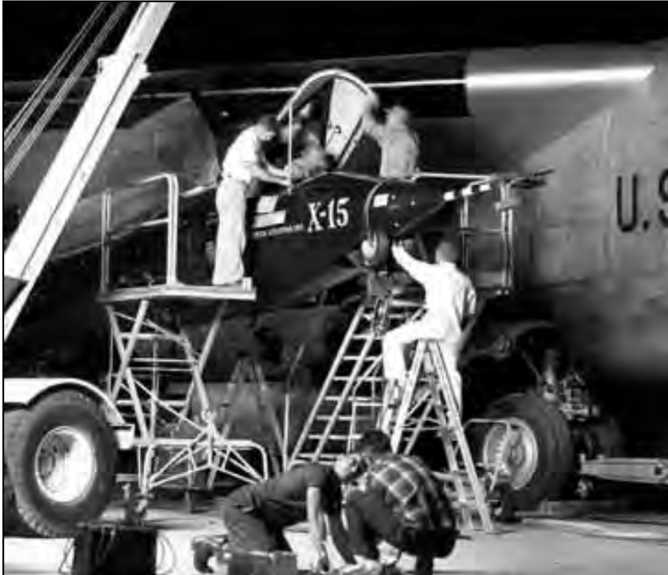
The early test flights were conducted with a long air data probe protruding from the nose of the X-15. Notice the technician manually retracting the nose landing gear on the X-15, something accomplished after the research airplane was firmly connected to the wing of the NB-52 mothership. (San Diego Aerospace Museum Collection)
