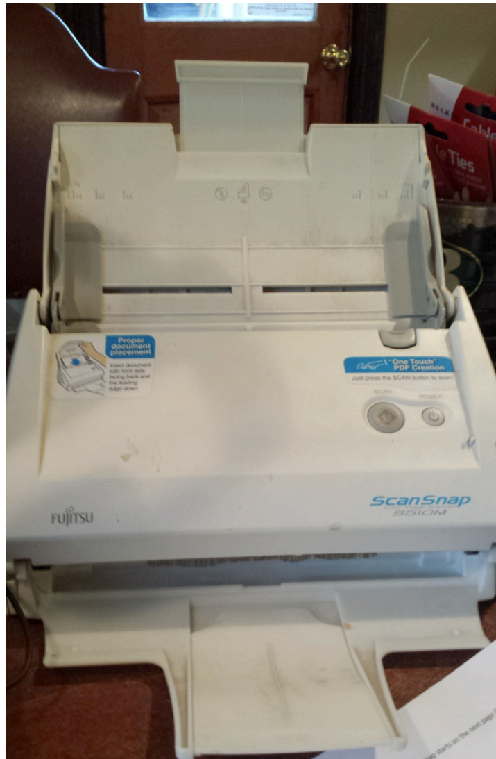
Example: A Fujitsu ScanSnap S510M sheet feed scanner, used by one of the IAPSOP principals. This device is the workhorse of our digitization efforts. This particular unit cost $495 in 2008, and has scanned more than 200,000 pages of printed material for IAPSOP, without a single service event.
