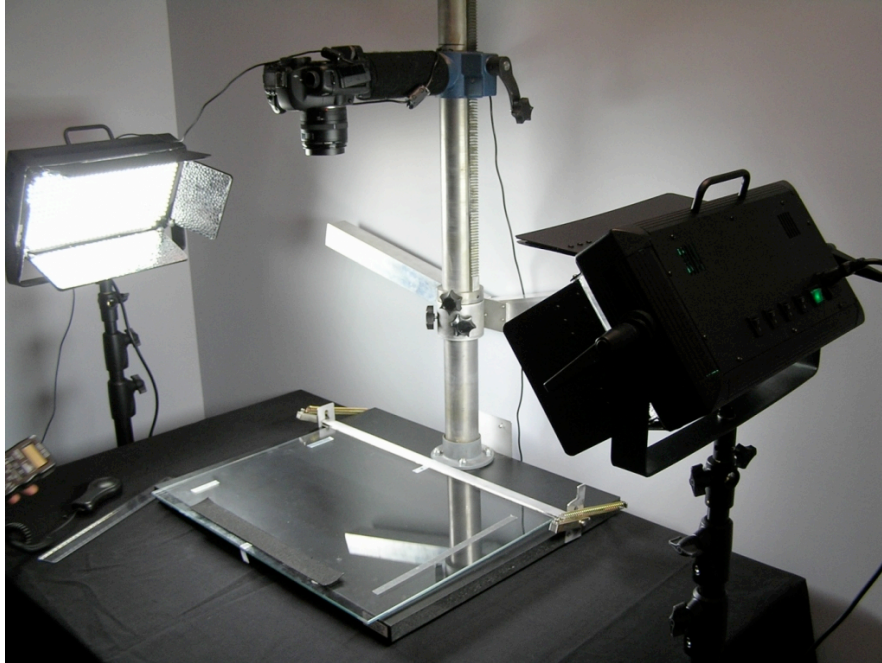
Example: A professional document camera rig, with a 13 megapixel Canon EOS digital SLR serving as the page image capture device. Similar, less expensive rigs, with light sources, are usually available from digital SLR camera manufacturers.
