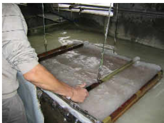
Fig. 15 Shaking mould front to back while water drains
