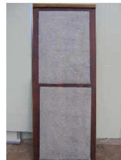
Fig. 21 Traditional method of drying sheets on wooden boards
