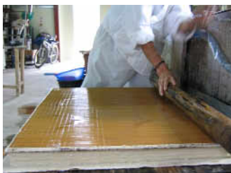
Fig. 18 Rolling log across post of wet sheets to remove bubbles
