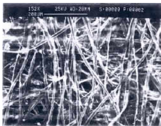
Fig. 22 SEM photograph of Dak fiber distribution in Webal formed paper (152X)
