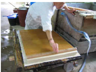
Fig. 17 Sheet is couching onto post of wet sheets
