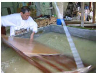
Fig. 10 Dipping left side of the mould into vat
