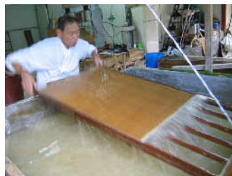
Fig. 9 Fibers flowing off the opposite side of the mould
