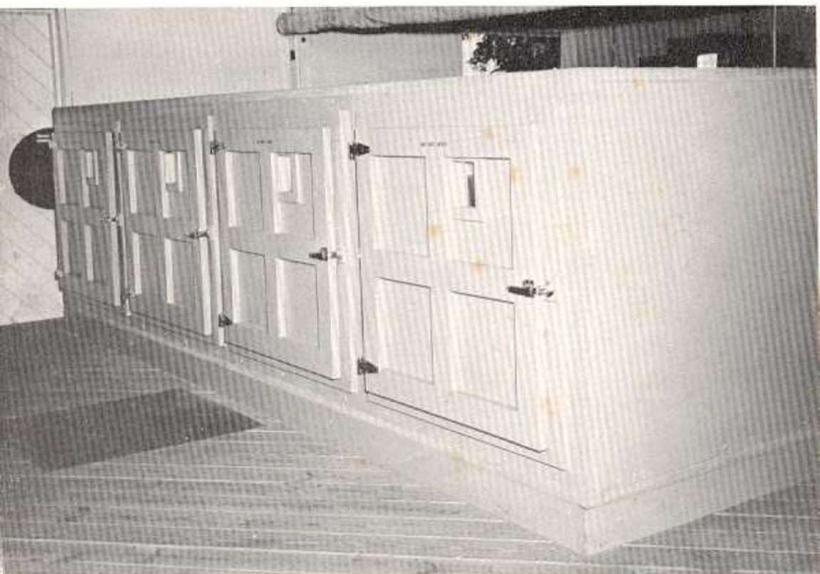
Fig. 1.—Degreening cabinets (approximately 50 cubic feet internal capacity each) used for small-scale experiments.
