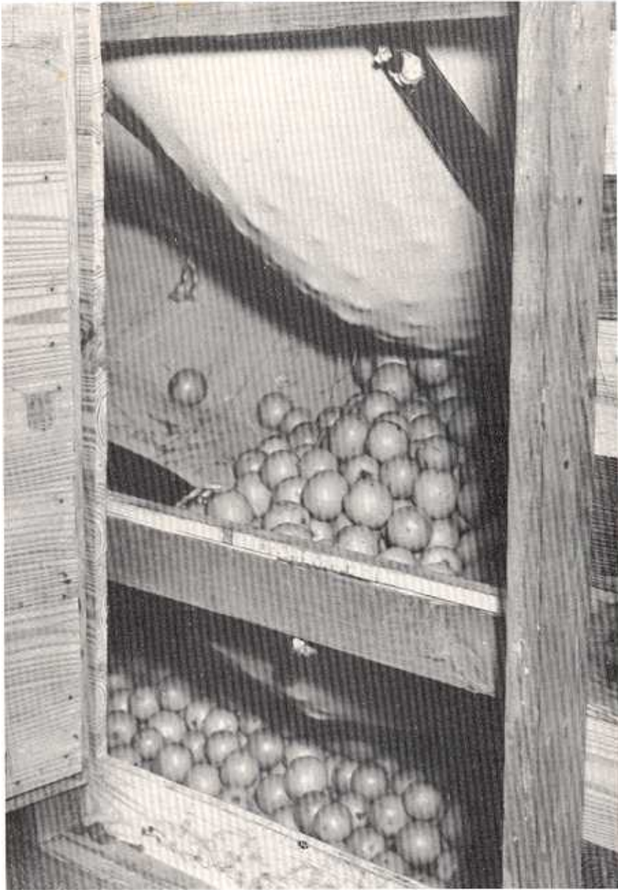
Fig. 12.—Interior of a bulk degreening bin in the process of being loaded. The lowest visible baffle is full and the fruit is starting to build up on the next baffle. The cloth used is soft and porous, allowing adequate air movement through the fruit. (See also Figure 11.)
