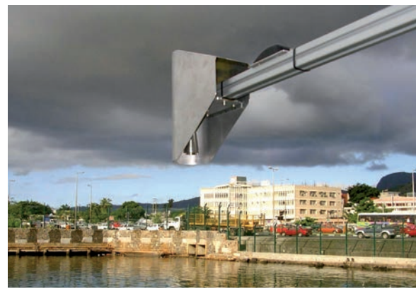
GLOSS sea level stations employ a number of instruments to measure sea level, including down-looking radars to measure sea level. Port Louis, Mauritius. Photo courtesy of University of Hawaii Sea Level Center.
