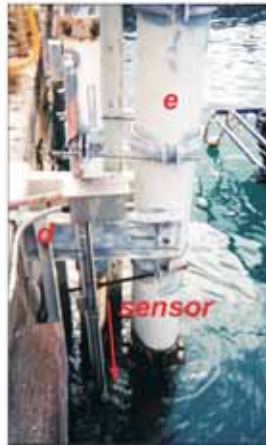
Rarotonga sea level station, Avarua Harbor, Cook Islands. The fiberglass electronics package (a), antenna (b), solar panel (c) were installed on a pier. Conduit (d) containing cables connecting the sensor, located at a depth of five feet below low-tide water level, to the data collection platform containing the electronics above, was externally attached to the tube containing the sensor (e).
