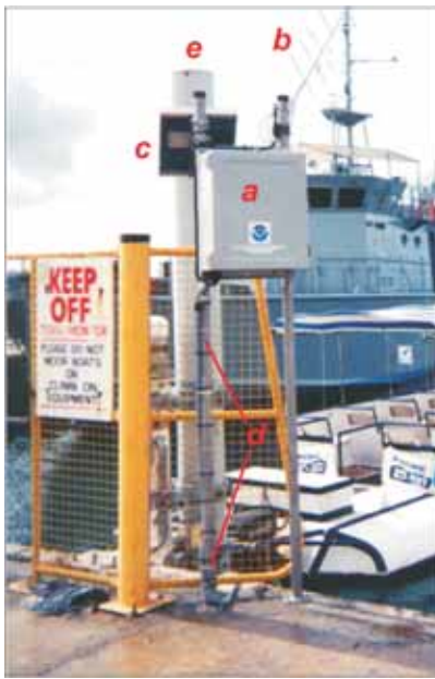
Rarotonga sea level station, Avarua Harbor, Cook Islands. The fiberglass electronics package (a), antenna (b), solar panel (c) were installed on a pier. Conduit (d) containing cables connecting the sensor, located at a depth of five feet below low-tide water level, to the data collection platform containing the electronics above, was externally attached to the tube containing the sensor (e).
