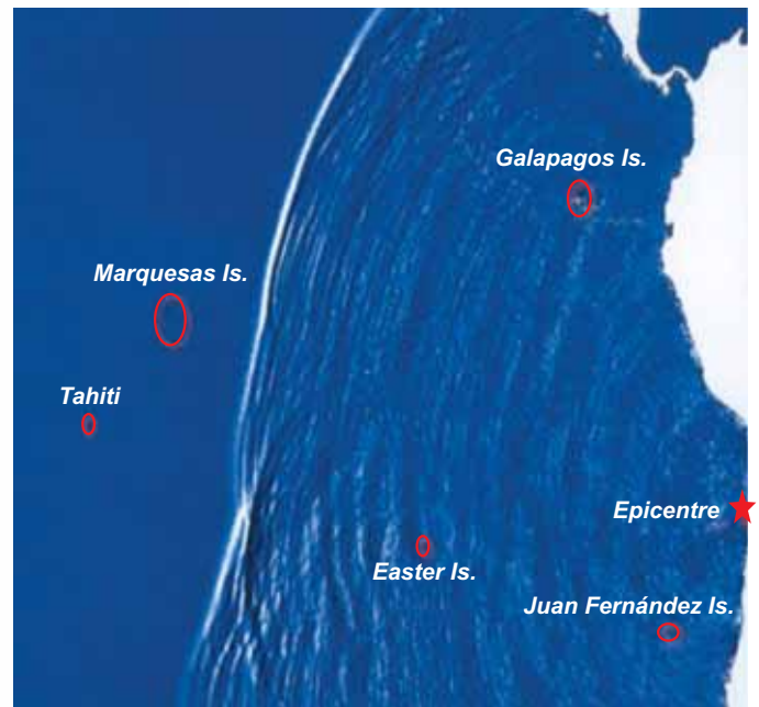
Model of tsunami propagation in the southeast Pacific, nine hours after generation. Source: Antofagasta, Chile (30 July 1995). Courtesy of LDG-France.
