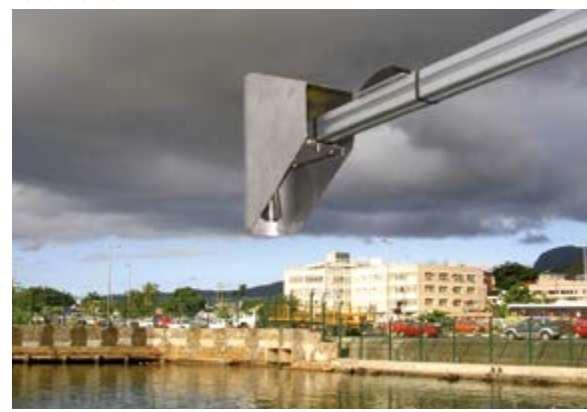
GLOSS sea level stations employ a number of instruments to measure sea level, including down-looking radars to measure sea level. Port Louis, Mauritius. Photo courtesy of University of Hawaii Sea Level Center. Courtesy of University of Hawaii Sea Level Center.
