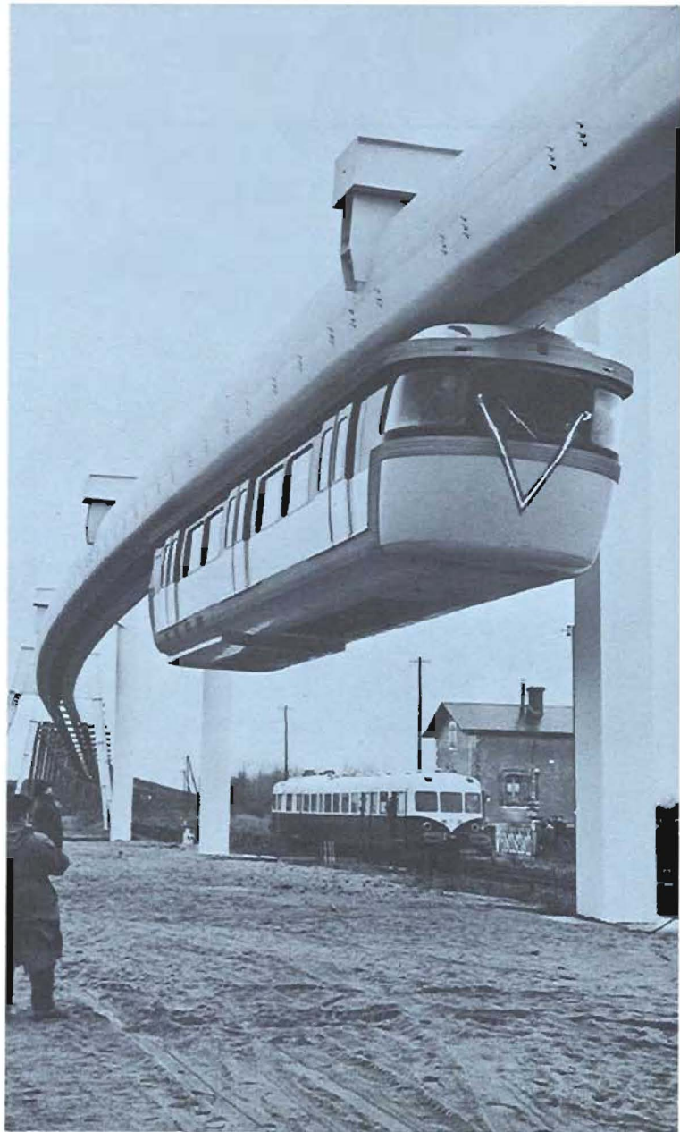
Suspended duorail train — S.A.F.E.C.E. test track near Paris
