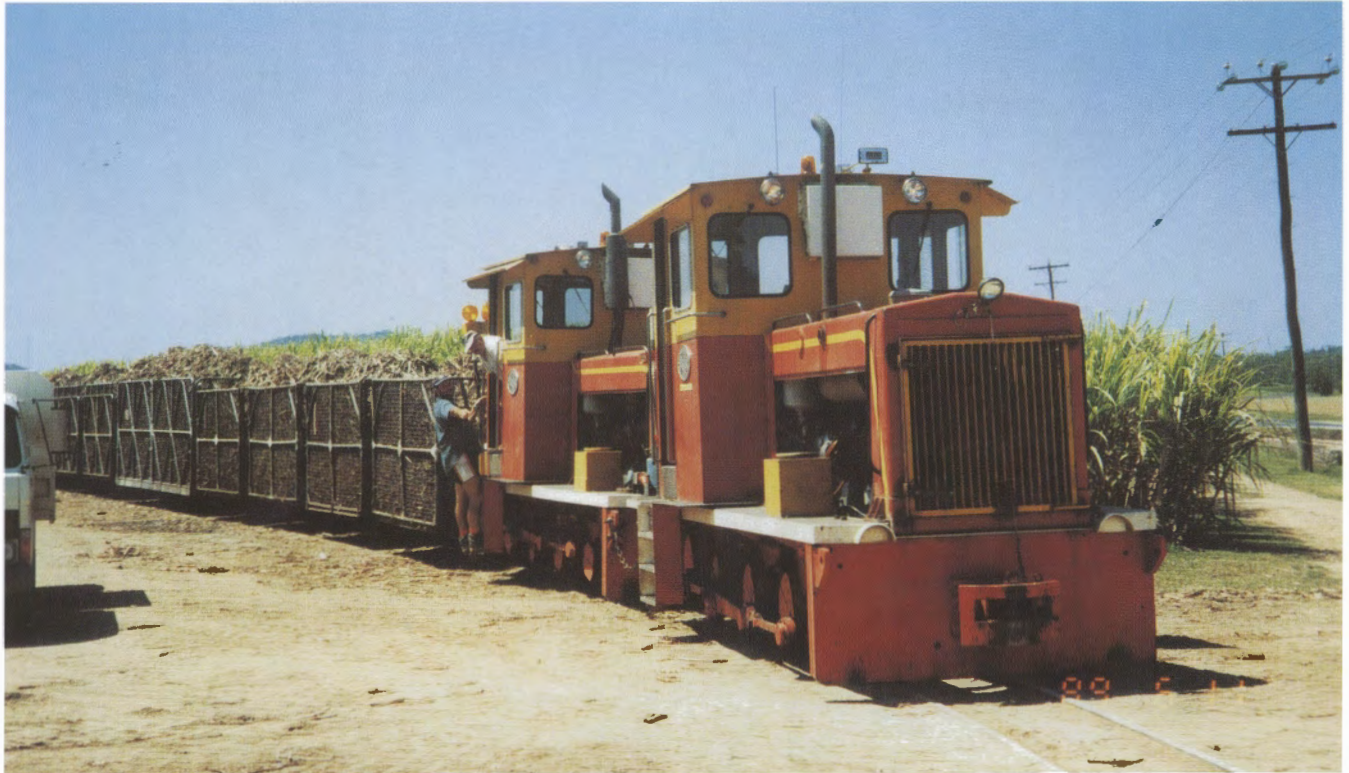
Com-Eng 0-6-0DH locomotive twins TULLY No. 14 (AK2663 of 1963) and TULLY No. 10 (AD1341 of 1960) haul cane from a spur siding just west of Birkalla during the 1997 season. Note the 11-tonne capacity bins in the train. Photo: Rod Milne
