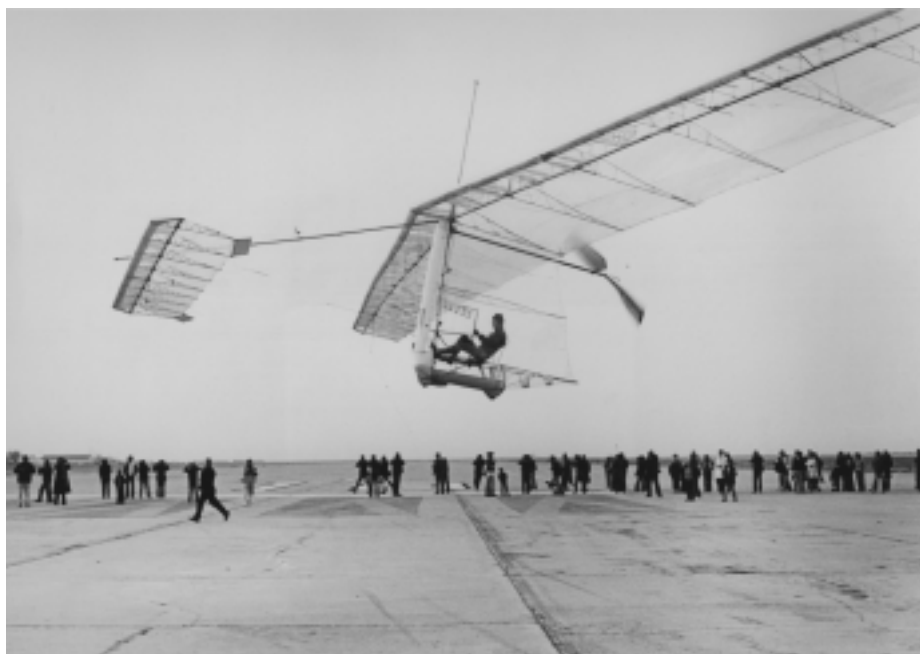
Figure 1.10 The world's first sustained flight powered by renewable energy in the form of food for humans. On August 23, 1977, the Gossamer Condor flew a distance of 1.3 miles in under seven minutes in a figure-eight pattern around two markers a half mile apart. It was powered by Bryan Allen, who provided the one-third horsepower required for the flight.
