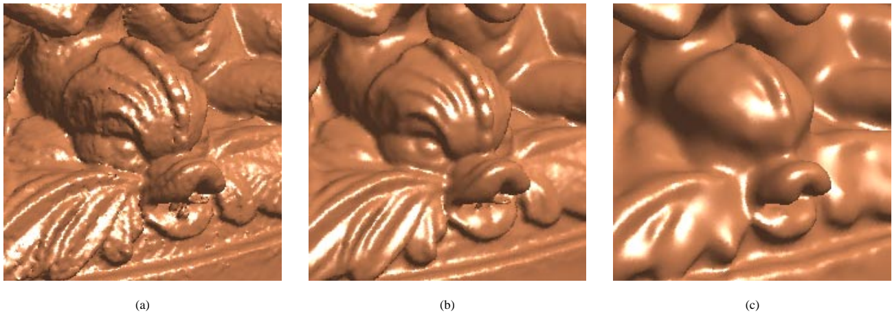
Figure 9: (a) Exact fit, (b) medium amount of smoothing applied (the RBF approximates at data points), (c) increased smoothing.
