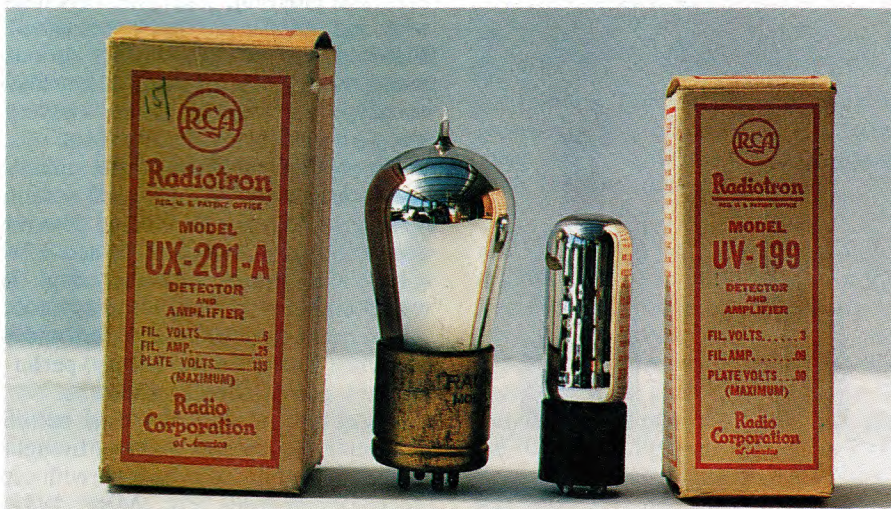
During the early and mid 1920's, the American scene was dominated by the '01A and '99. In contrast with the pure tungsten filament valves, these thoriated tungsten types needed heavy gettingter.
