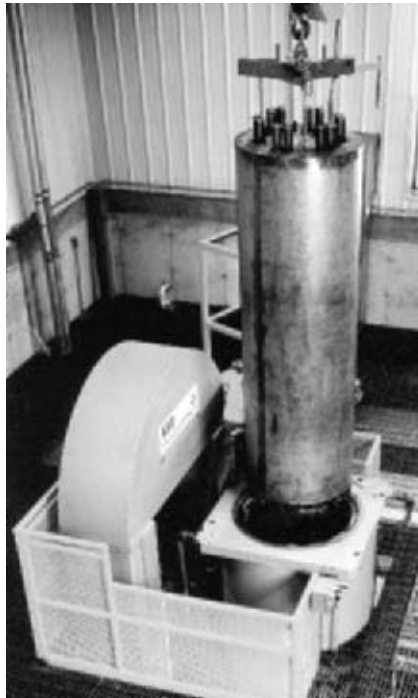
Figure 8.43: Hot Isostatic Press, Commercial. HIPs of various sizes, temperature, and pressures are available. (Courtesy of ABB Autoclave)
