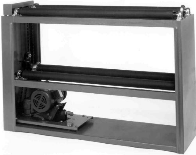
Figure 3.15: Commercial Mill Rack
