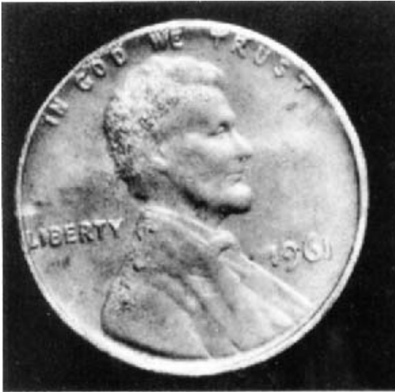
Figure 8.42: Coined Alumina Penny. By pressing graphite powder over a contoured face, a reproduction can be made with a ceramic part.
