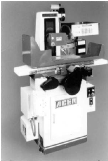
Figure 9.5: Surface Grinder. Grinding machines should be rigid and dampen vibrations. (Courtesy of Chand Kare)
