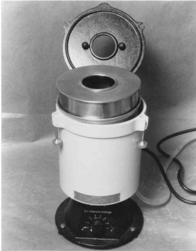
Figure 4.23: Decanting Centrifuge. Slip enters into the bottom by a peristaltic pump. Fines are taken off up the shell and can be recirculated to remove additional coarser particles. (Courtesy of IEC).
