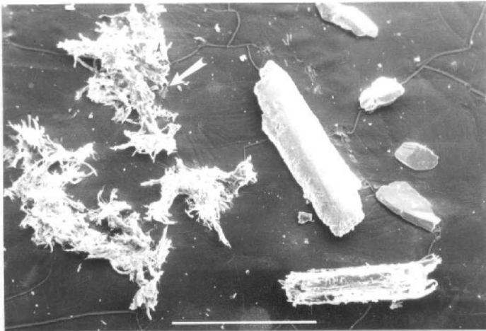
Figure 4.25: Debris Recovered from a Slip by Filtering. Even a high purity slip can contain extraneous material.
