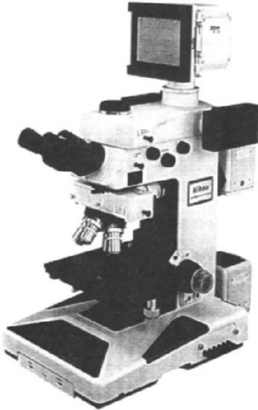
Figure 11.27: Universal Microscope. Used for reflected, transmitted, and oblique illumination. (Courtesy of Nikon)
