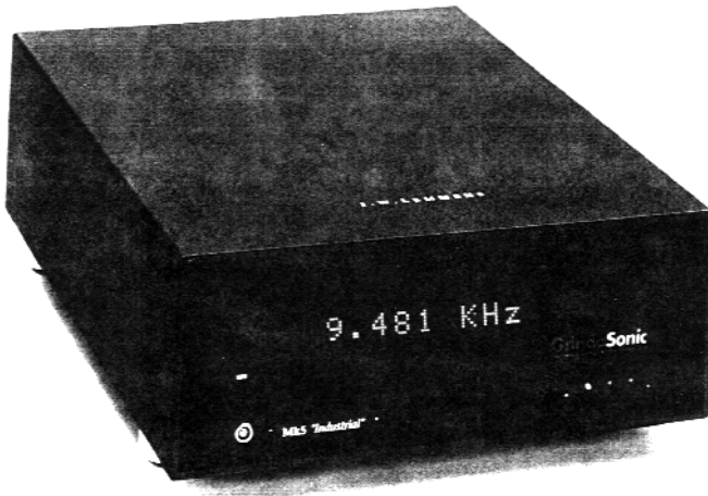
Figure 11.72: Resonate Frequency Measurement Apparatus for MOE measurements. Easy to use. (Courtesy of Grindosonic/Lemmings)
