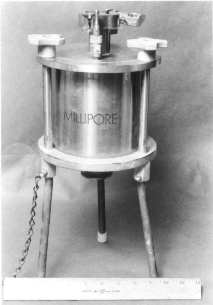
Figure 4.22: Pressure Filter Apparatus. The filter is used to remove extraneous material. (Courtesy of Millipore).
