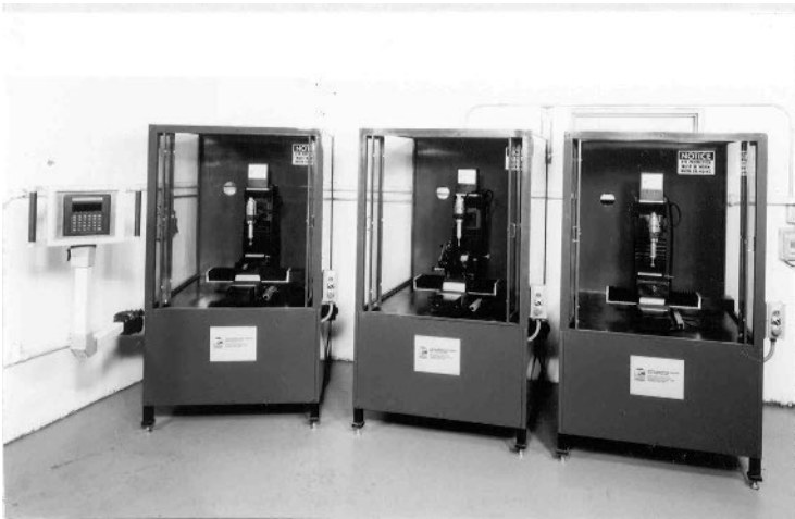
Figure 7.8: Green Machining Center. Commercial green machining centers that feature abrasive cutting tools are available. (Courtesy of Chand Kare)
