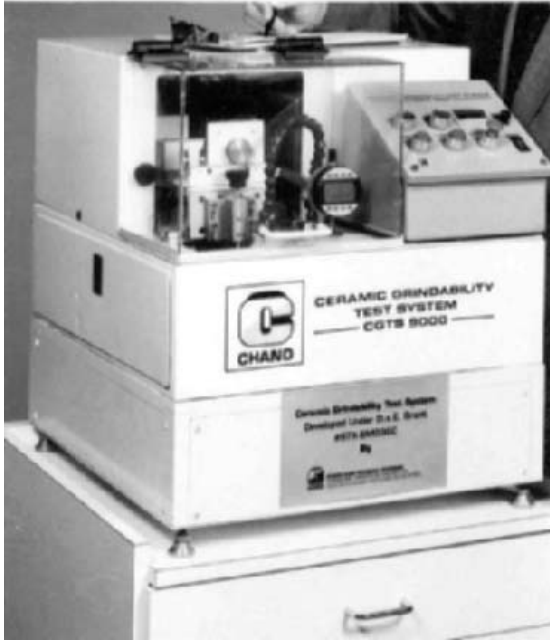
Figure 9.6: Grindability Test System. The test results help in selection of wheel specifications and grinding conditions. (Courtesy of Chand Kare)
