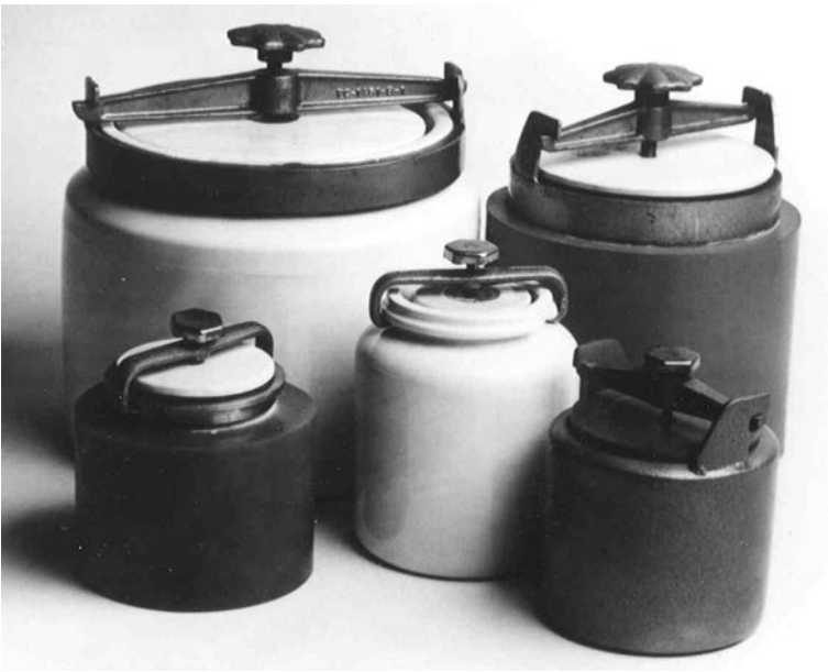
Figure 3.1: Typical Alumina Fortified Jar Mill (courtesy of E.R. Advanced Ceramics).
