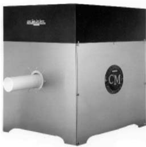
Figure 8.7: Tube Furnace, Commercial. Tube furnaces are available in a variety of sizes and temperature capability. (Courtesy of CM Furnaces).
