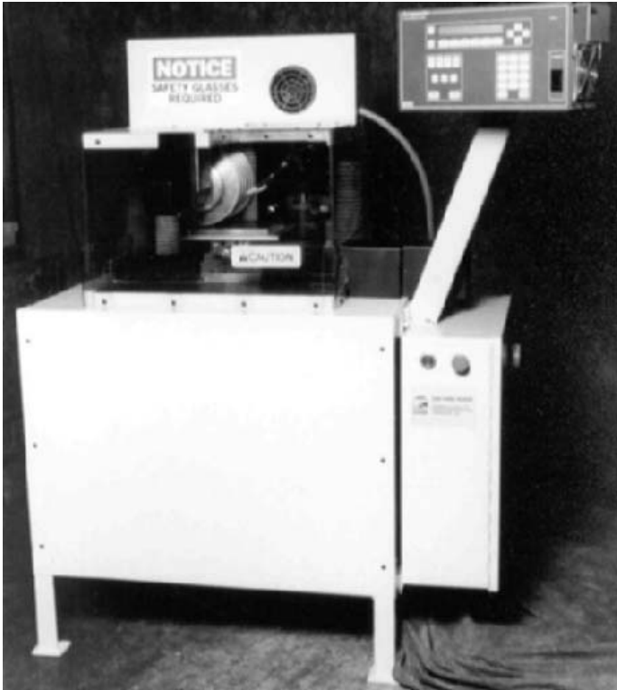
Figure 9.7: Cutoff/Gang Slicer. Multiple cuts with ganged wheels speed up the cutoff process. (Courtesy of Chand Kare)
