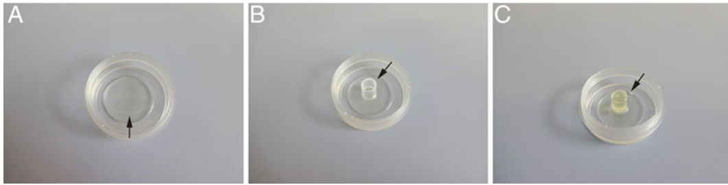
Fig. 2 (a) Glass-bottom cell culture dish. It was filled with EPON embedding medium at the central area which is confined by the glass cover slip (arrow). In (b) a BEEM capsule was placed on the cover slip (arrow) and filled up with EPON embedding medium (c) (arrow)
