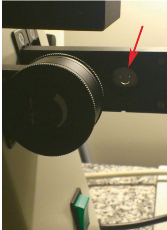
Fig. 2 The mechanical shutter and sliding filter holder of a microscope can be used to introduce a thin prefabricated metal plate (here: smiley face; red arrow ) for patterned illumination of the biological sample (Color figure online)
