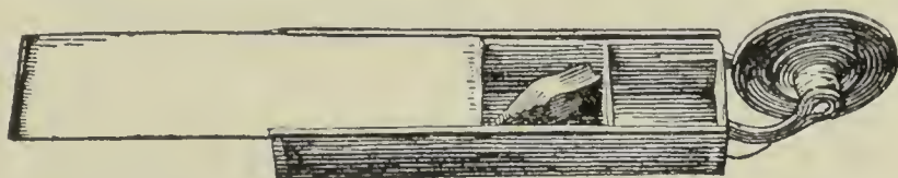
Wheel-tinder-box of tin (japanned), with three compartments and a steel wheel.
