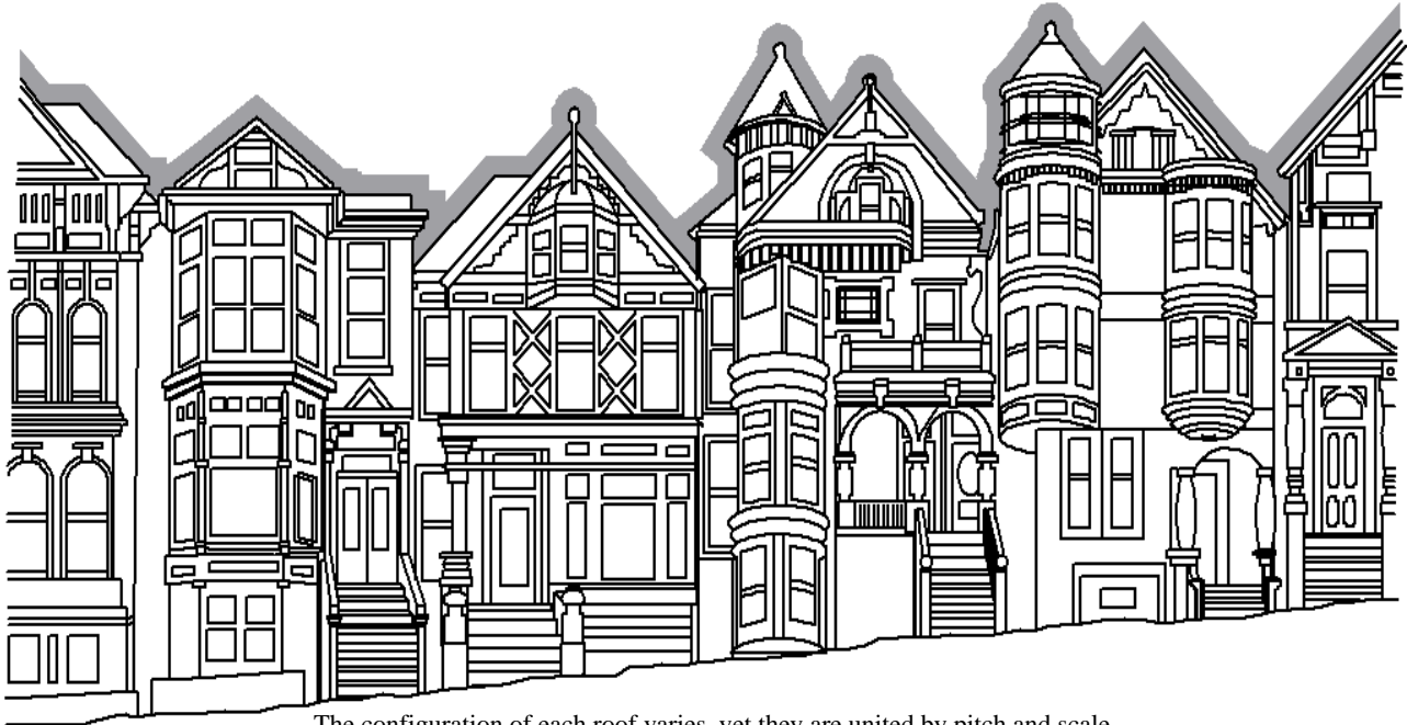
The configuration of each roof varies, yet they are united by pitch and scale.
