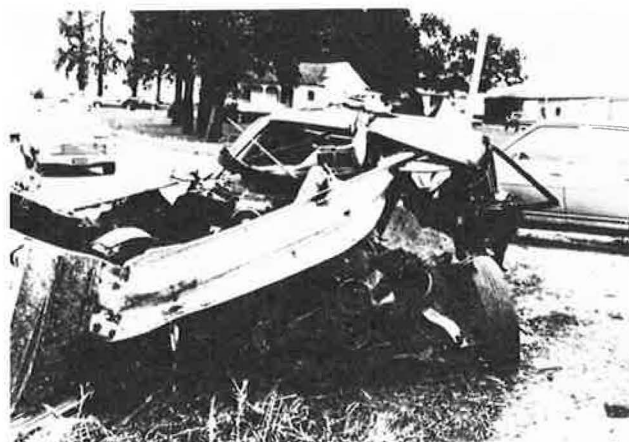
FIGURE 1 Unprotected or unmodified guardrail ends are lethal roadside hazards.
