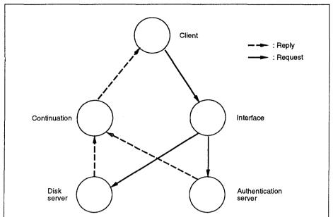
Fig. 9. Topology of the request-reply communication between the interface, continuation, authentication, and disk servers.
