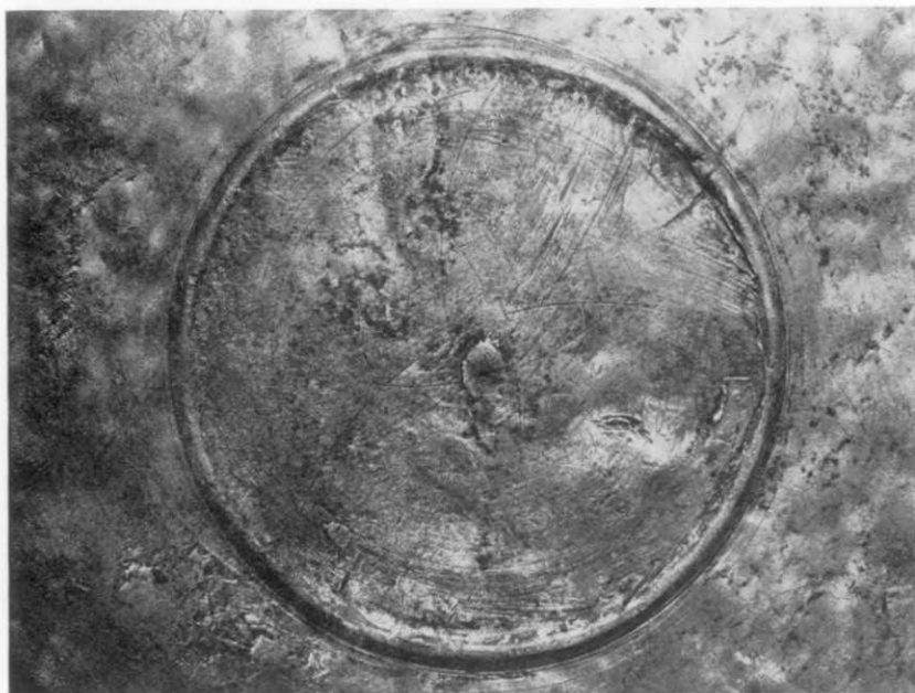
A. The back of plate 12 showing compass work and lathe mounting scars.
