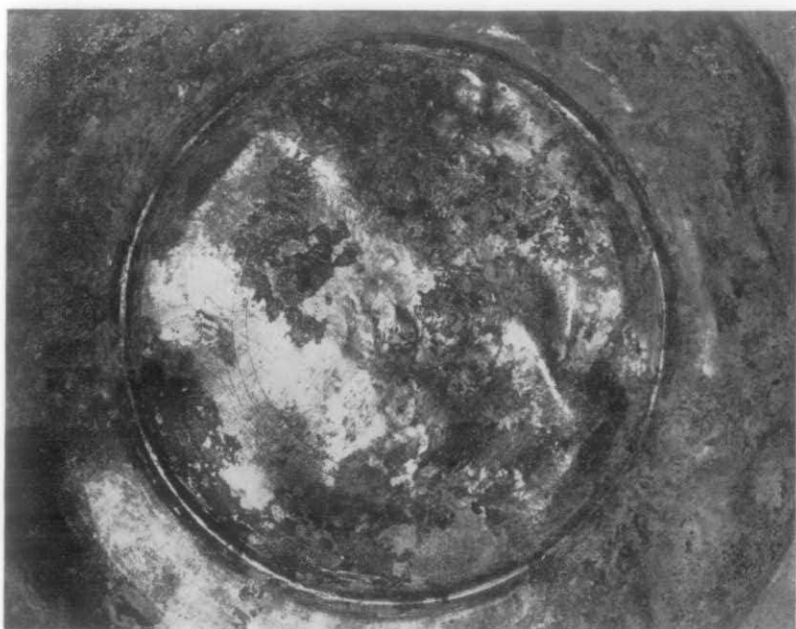
A. The back of plate 17 showing typical compass work and lathe mounting scars.
