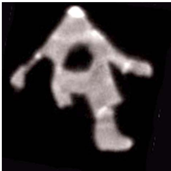
Figure 3. Animation of neutron attenuation through an axis (No. H25-1) of an undetermined diplodocid sauro-pod. Like Figure 2, the movie is composed of axial slices from cranial to caudal regions, taken through the vertebra. For the left lateral view of No. H25-1 see Figure 4a. Green scale bar below the object is 10 cm.
