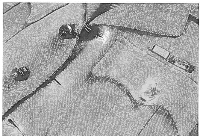
Figure 12. Mould often becomes visible as whitish spots, but other colours are common. Here mould is growing supported by the nutritional value of the oils on the leather buttons.
