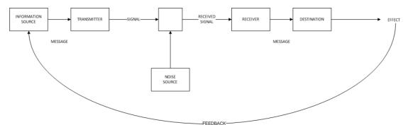
Figure 2-3 Shannon's schematic diagram of a general communication system with feedback added
