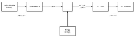
Figure 2-2 Schematic diagram of a general communication system (Source: Shannon, 1948)
