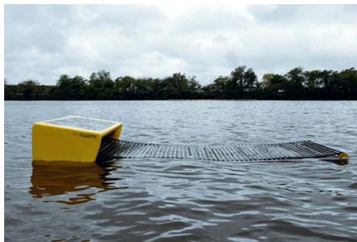
Figure 5.14. “Seaswarm” is a nanotechnology-enabled oil-spill-cleaning robot developed by a group of MIT engineers ( TechNews Daily , August 25, 2010). The conveyor belt of the robot is coated with a mesh of superhydrophobic nanowires developed by Yua et al. (2008).
