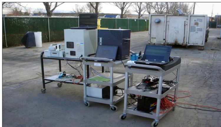
Figure 4.8. Example of field application of instruments needed for real-time measurement of number, mass, size distribution, and surface area of engineered nanomaterials (courtesy of A. Nel).
