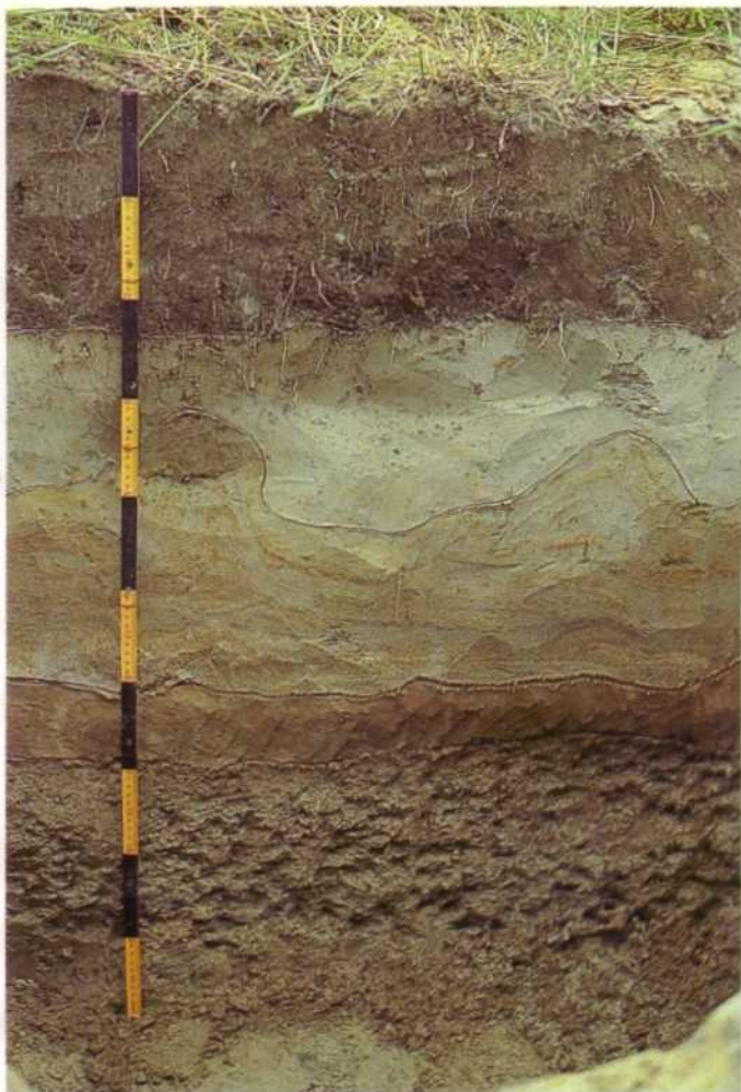
Figure 25. Manotick association soils feature 40 to 100 cm of sandy material overlying clays. Soils ranging from well to very poorly drained were included in this soil association. This example is a poorly drained Orthic Humic Gleysol (Allendale series) featuring an A horizon rich in organic matter and subsurface horizons which are heavily mottled.
