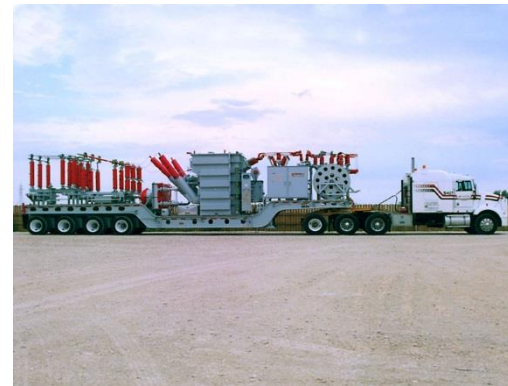
HV Power Fuses on rear of Trailer
