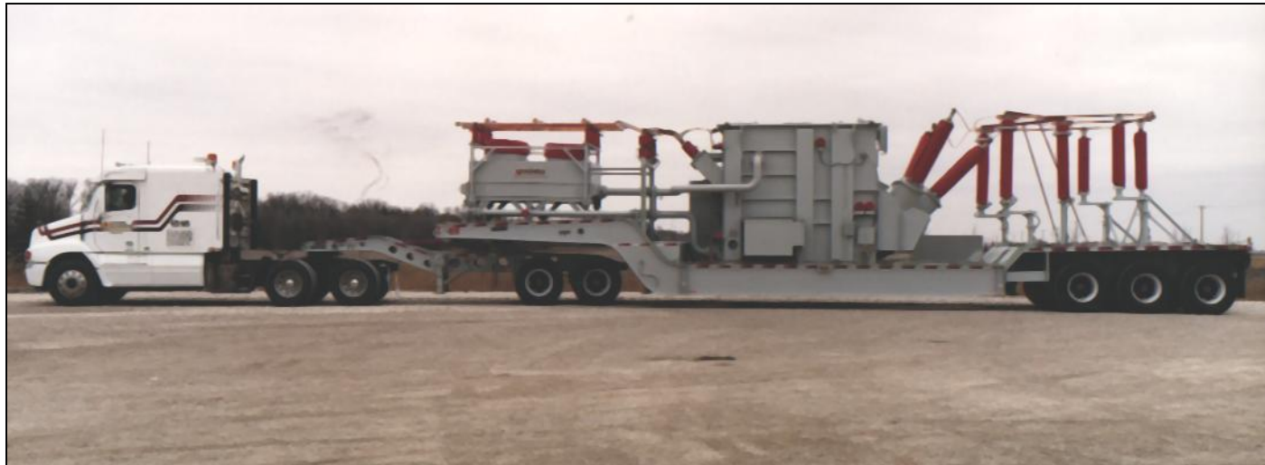
40 MVA, 161.7 - 13.09 x 26.18kV 95°C. Winding Rise
