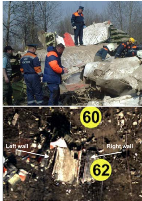
Figure 15. Left and right walls cut off from fuselage on 04.11.2010. Separated walls (white arrows) on air photo in IAC report.
