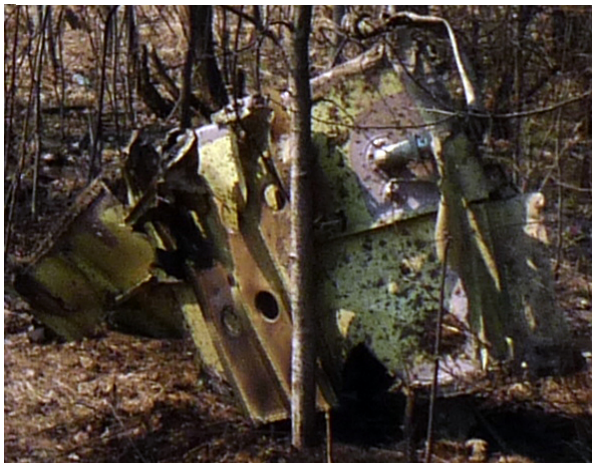
Figure 28. The aircraft's center wing box around 80 m in front of main center wing position on the crash site. On the surface visible signs of the fire.
