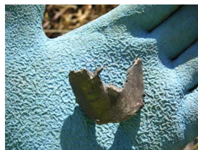
Figure18. Example of a burned metal piece of debris found in front of main crash site. Appendix XI.
